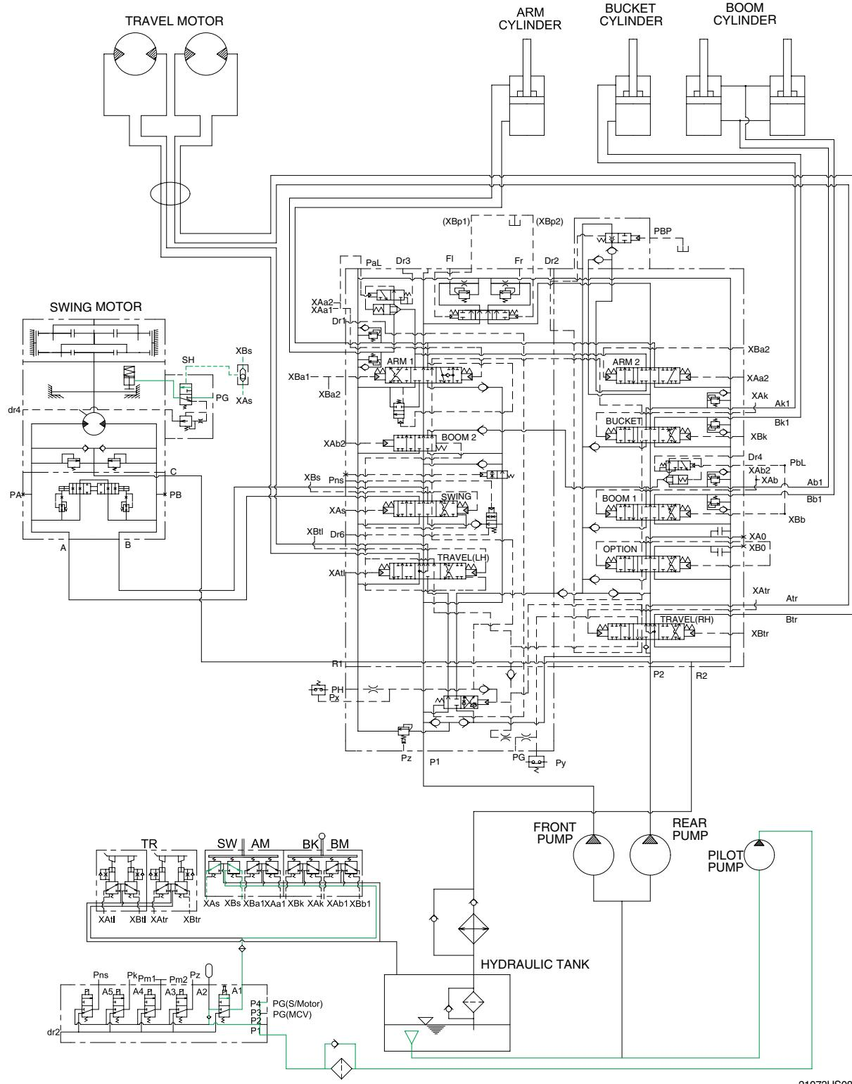
When the swing control lever is tilted, the pilot oil flow into SH port of shuttle valve, this pressure move spool so, discharged oil from pilot valve flow into PG port.
