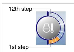
(1) This gauge indicates the temperature of coolant in 12 step gauge.
