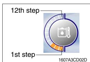
(1) This gauge indicates the temperature of hydraulic oil in 12 step gauge.
