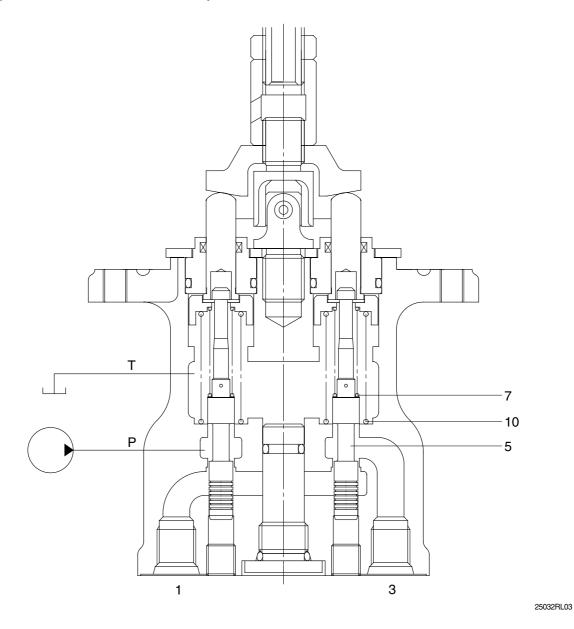
The force of the spring(7) that determines the output pressure of the pilot valve is not applied to the spool(5). Therefore, the spool is pushed up by the spring(10) to the position of port(1, 3) in the operation explanation drawing. Then, since the output port is connected to tank port T only, the output port pressure becomes equal to tank pressure.
