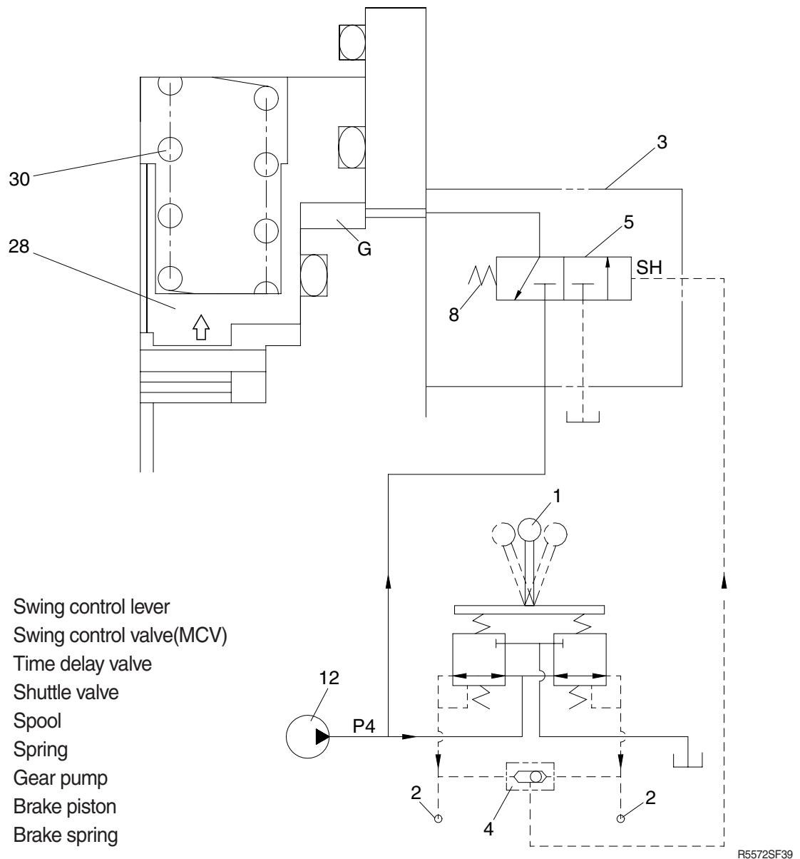
b. When the swing control lever(1) is set the neutral position, the time delay valve(3) shifts the neutral position and the pilot oil blocked chamber G.
