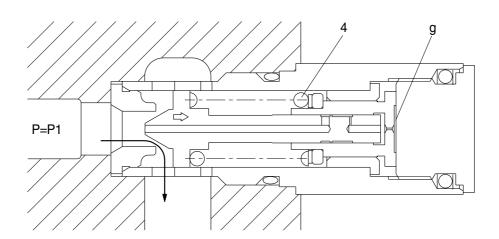
③ The oil flow chamber g via orifice m and n. When the pressure of chamber g reaches the preset force(FSP) of spring(4), the piston(6) moves left and stop the piston(6) hits the bottom of bushing(7).
