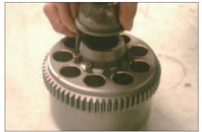
② Put piston (121), shoe (122) subassembly in set plate (123) and then assemble them to cylinder block (111).
