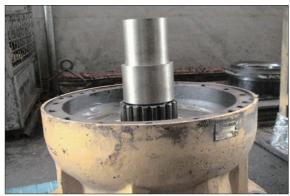
③ Remove roller bearing (6) from gear casing (1).
