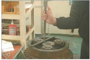
(19) Measure height "B" from side cover (4) mating face to center hold bottom with straight edge and depth gage.
