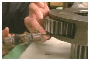
(14) Screw two M10 eyebolts into carrier 2 sub-assembly, and assemble it with crane, paying attention to its meshing with planetary gear 2 and ring gear.
