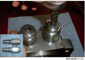
③ Disassemble make up check valve assy with a torque wrench from rear cover (23).
