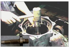
5 Fix snap ring (4) to shaft with a plier jig.  $\cdot$  Snap ring  $\times 1\text{EA}$
