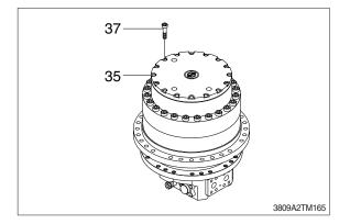
(26)Inject gear oil and assemble plug (41) of cover (35).
