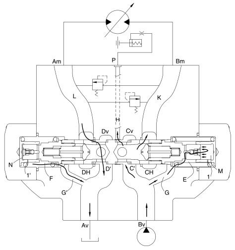
Suppose port Bv is connected to the hydraulic pump and Port Av, to the tank. The oil supplied from the hydraulic pump passes through Bv, Cv and C' in sequence, pushes up the poppet of the check valve, passes through K to Port Bm, and is supplied to the hydraulic motor to turn it.
