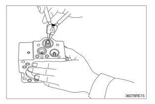
(11) Fit set spring (655) to spool hole and put compensating piston (621) and piston case (622) into compensating hole.Fit pilot cover (641) and tighten it with hexagonal socket head screws (436, 438).
