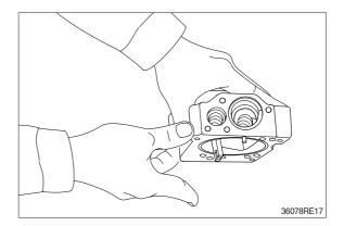
(13) Install cover (C, 629) fitted with adjusting screws (628, 925), adjusting stem (C, 627), lock nut (630), hexagon nut (802) and set screw (924).
