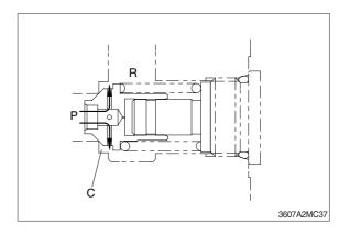
③ When the pressure in the path (P) goes over the set pressure of the spring(621), the poppet (611) opens. Then, the pressurized oil in the path (P) passes around the outside of the poppet (611) and flows to the low-pressure path (R).
