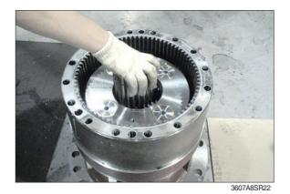
(8) Assembly of sun gear 1, carrier 1 assembly
