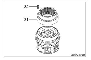
(13)Remove hub (3) from assembly (1). - Tools : I-bolt, Hoist
