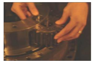
(10) Insert pin 3 (17) into shaft casing, and then assemble snap ring (37).
