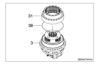
(14) Tighten hub and ring gear.
