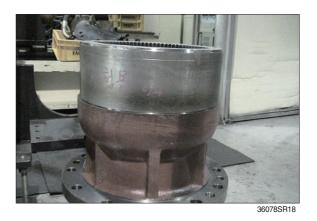
(6) Assembly of carrier 2 assembly
