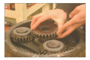
(18) Measure height "A" from sun gear 1 end face to ring gear (1) mating face with straight edge and depth gage.
