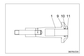
Remove rod packing (9), back up ring (10) and dust seal (11).
