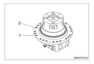
(2) Assemble thrust plate (15) to spline surface of track motor (1).
