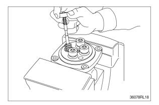
(5) Assemble O-ring (15) onto plug (14).
