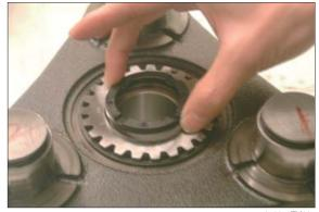
④ Put needle cage (21) into inside of planetary gear 1 (12), and assemble them, holding them between side plates (18). Then fit snap ring (44) on them.
