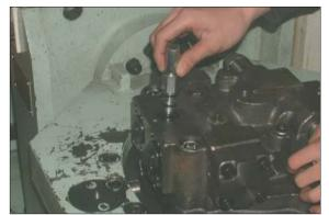
③ Remove plug (564) from valve casing (303). And then screw two M10 $\times$ 135 bolts on the holes of compelling brake release. Sub assembly (valve casing & brake piston)
