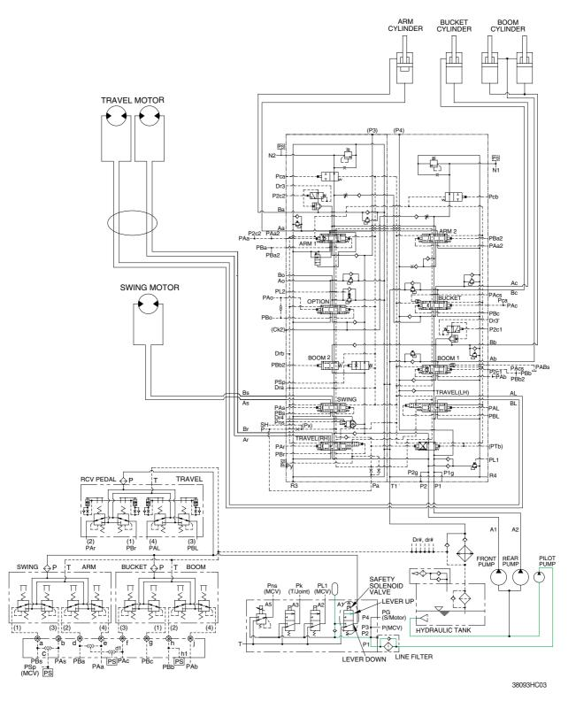
When the lever of the safety solenoid value is moved downward, oil flows into the remote control value through solenoid value and line filter.
