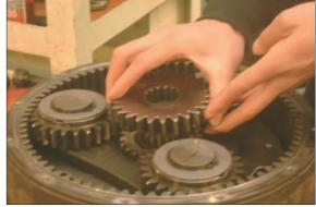
(6) Remove carrier 1 (5), together with planetary gears 1 (12), sun gear 2 (10), etc. fitted.
