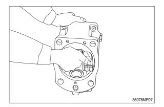
(13) Tapping lightly shaft ends of drive shafts(111, 113) with plastic hammer, take out drive shafts from swash plate supports.
