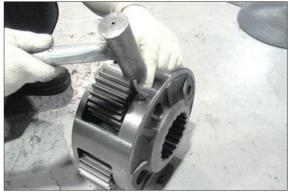
② Remove pin assy 2 (11) from carrier 2 (7), planetary gear 2 (9) and thrust washer (14) with hands.
