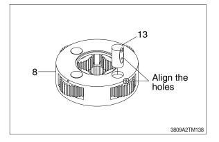
④ Assemble carrier (8) and pin (13) striking pin (14) by hammer.
