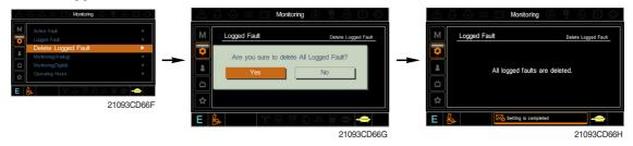
• The logged faults of the MCU or engine ECM can be deleted by this menu.
