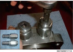
$\ensuremath{\textcircled{}}$  Disassemble make up check valve assy with a torque wrench from rear cover (23).
