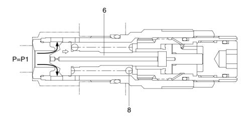
③ When the pressure of chamber g reaches the preset force(Fsp) of spring(8), the piston(7) moves right and stop the piston(7) hits the end of body.
