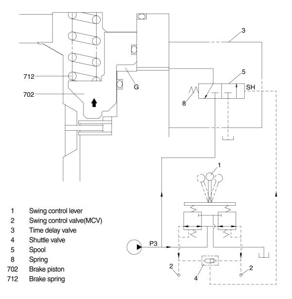
b. When the swing control lever(1) is set the neutral position, the time delay valve(3) shifts the neutral position and the pilot oil blocked chamber G.
