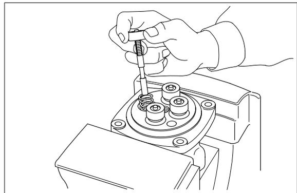
(5) Assemble O-ring(13) onto plug(11).
