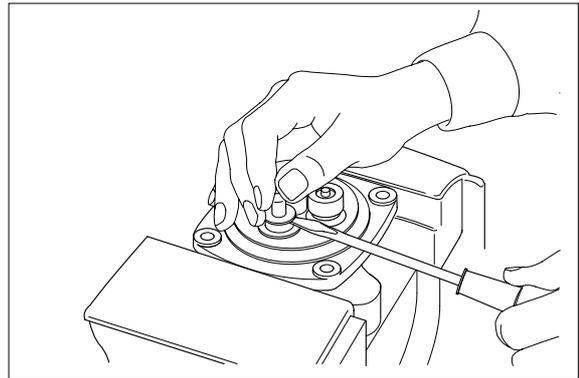
(9) Remove reducing valve subassembly and return spring(10) out of casing.
