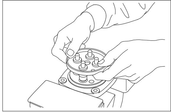
(8) When return spring(10) is weak in force, plug(11) stays in casing because of sliding resistance of O-ring.
