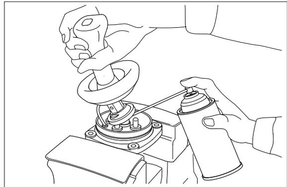
(19) Assemble lower end of bellows to casing.
