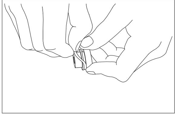
(6) Assemble seal(12) to plug(11).
