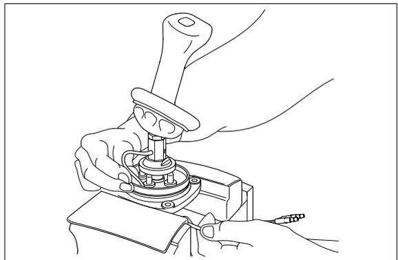
(17) Determine handle direction, tighten lock nut(20) to specified torque to fix handle.
