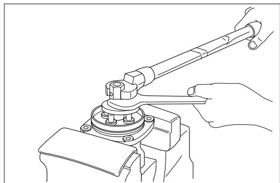
(14) Fit boot(25) and lock nut(20), and handle subassembly is assembled completely.
