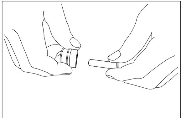
(8) Assemble plug subassembly to casing.
