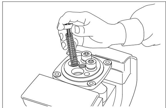
(10) Loosen hexagon socket head plug(2) with hexagon socket screw key.
