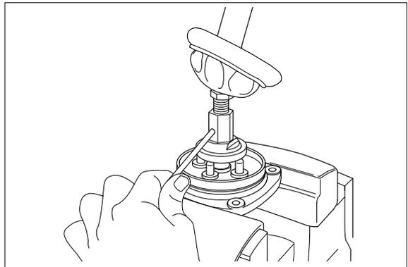
(16) Assemble bushing(16) to plate and pass cord and tube through it. Provide margin necessary to operation.
