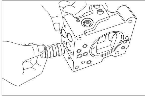
(12) Put spring seat(644), pilot spring(646) and adjusting ring(Q, 645) into pilot hole.
