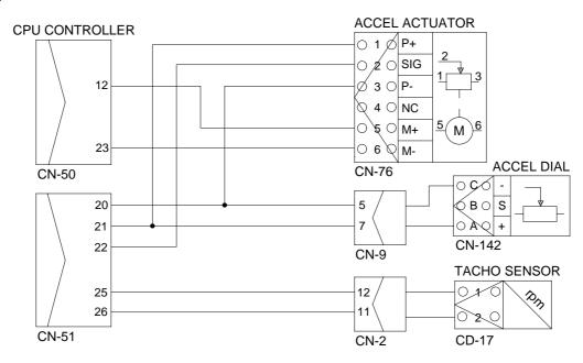
(1) **Test 5**: Check resistance between CN-50 (12)-(23).
