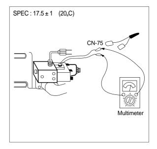
(3) **Test 3**: Check electric current at EPPR valve.
