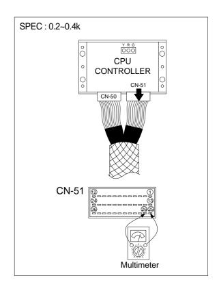
(4) **Test 8 :** Check resistance at speed sensor.
