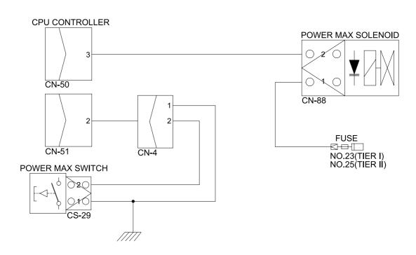
(1) **Test 15:** Check voltage between connector CN-88 - GND.
