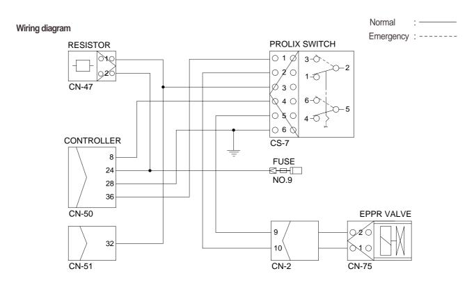
(1) **Test 1**: Check resistance at connector CN-50(8)-(36).
