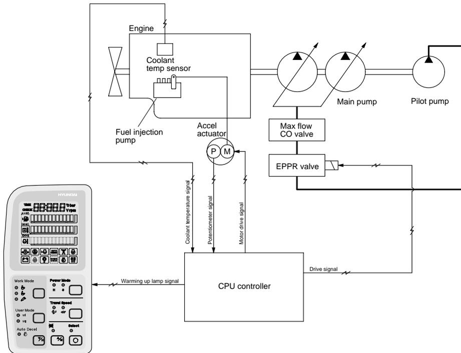
1. CPU controller reads engine coolant temperature through the temperature sensor, and if the coolant temperature is less than 30°C, it increases the engine speed from key start rpm to 1200rpm. At this time the mode does not change.
