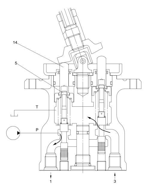
When the push rod(14) is stroked, the spool(5) moves downwards.
