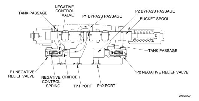
When no function is being actuated on P1 side, the hydraulic fluid from the pump P1, flows into the tank passage through the bypass passage and orifice. The restriction caused by this orifice thereby pressurizes. This pressure is transferred as the negative control signal pressure Pn1 to the pump P1 regulator.
