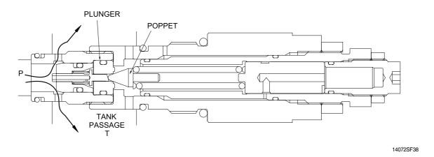
④ High pressure setting pilot signal(Pu) : ON
