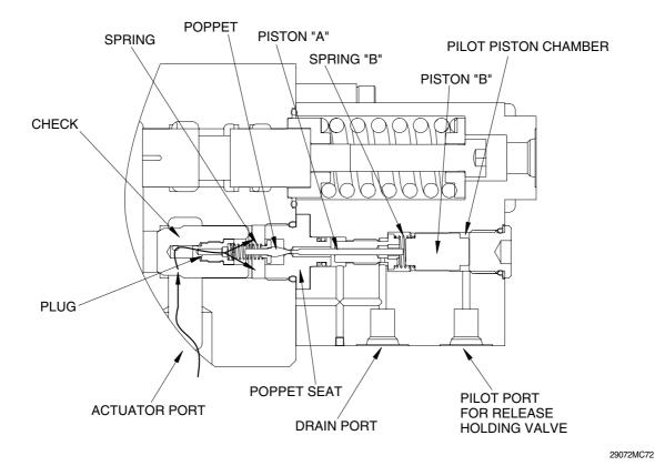
At neutral condition, the pilot piston chamber is connected to drain port through the pilot port.
