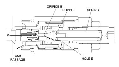
© Opening of the poppet causes the pressure in chamber A to fall and the plunger to open. As the result the pressurized oil at port P runs into tank passage (T).
