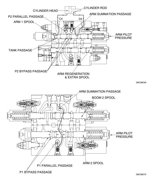
During arm roll out operation the pilot pressure from RCV is supplied to the port Pd40 and the Pd41 and shifts arm1 spool and arm2 spool in the right direction.
