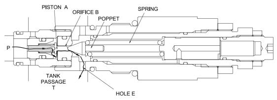
③ Opening the poppet causes the pressure in chamber A to fall and the plunger to open. As the result the pressurized oil at port P runs into tank passage (T)
