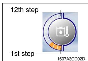
① This gauge indicates the temperature of hydraulic oil in 12 step gauge.
