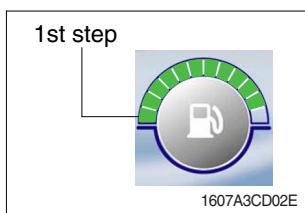
① This gauge indicates the amount of fuel in the fuel tank.
