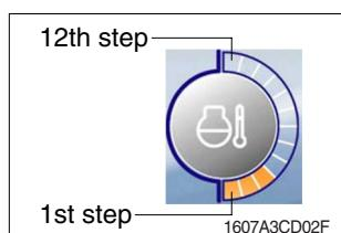
① This gauge indicates the temperature of coolant in 12 step gauge.
