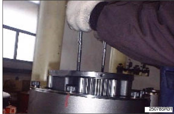
Moue out ring gear by the removal groove between ring gear(22) and casing(1) by using removal jig.
