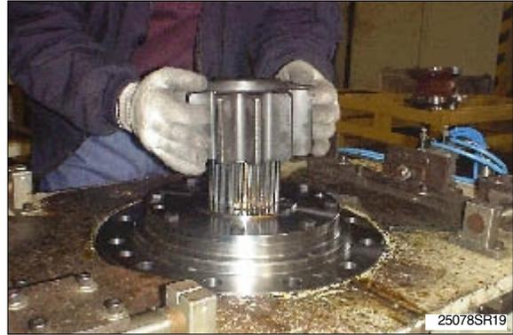
Put lock plate(26) and lock washer(27),
