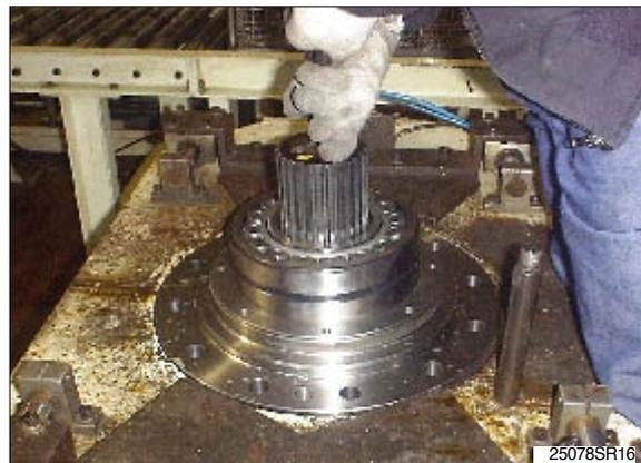
Assemble cover plate(5) and thereafter spacer(3).
