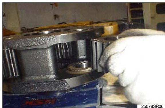
Place No.2 planet gear(11) onto the right location of the carrier(9).
