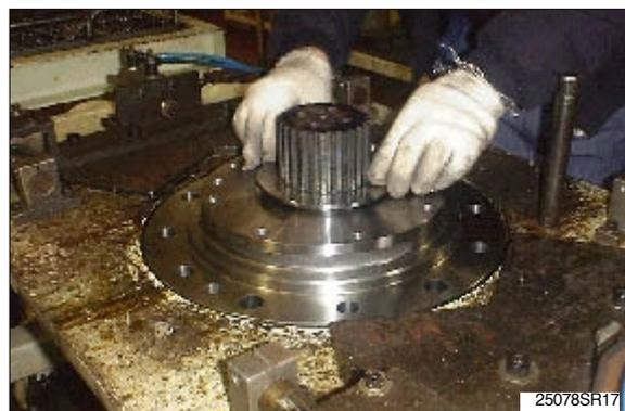
Assemble cover plate(5) with case(1) after spreading loctite 262 and tighten hex bolt(M10) (6).
