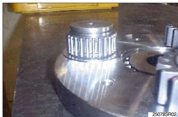
Put No.1 planet gear(18) and No.2 side plate(31) together and install a stop ring(32) by using assembling.
