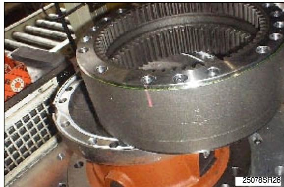
Place ring gear(22) on the case by matching knock pin hole.
