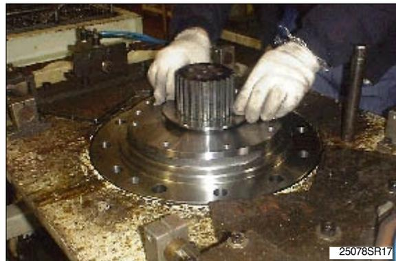
Dismantle drive shaft by using jig
