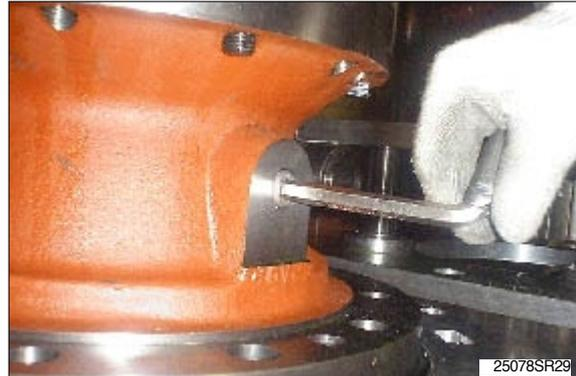
Loosen the socket bolts(24) to separate swing motor from reduction gear.
