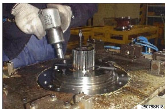
Install pinion gear(25).
