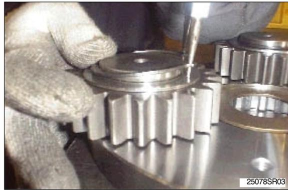
Insert spring pin(33) into the carrier sub-assembly by using jig and hammer.
