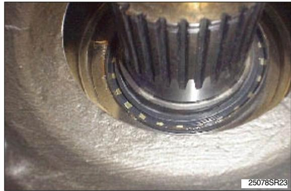
Spread loctite 609 on the outside ring of roller bearing(8) and insert the bearing(8) by using a pressing jig.
