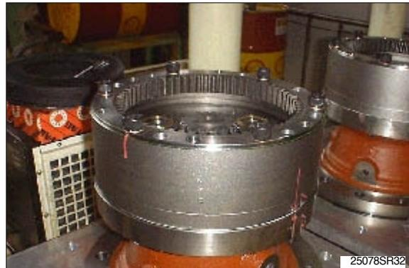
Mount No.1 carrier assembly in the case sub assembly and install bolts into 2 tap holes(M8).
