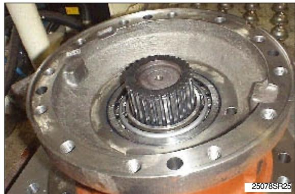
Clean the assembling surface of case and spread packing liquid(TH1105).
