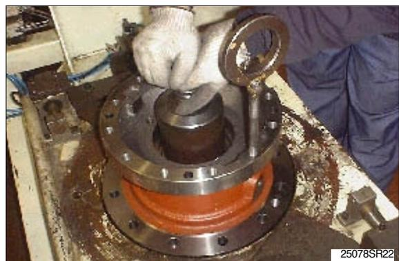
Be sure to check by eye the oil seal(7) is seated completely after being installed.
