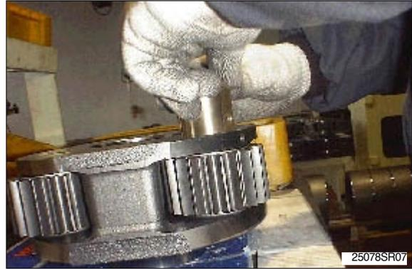
Assemble the planet gears(11) and carrier (9) by inserting the pin assembly(12) using rubber hammer. Pay special attention to locate the spring pin hole to meet with the hole of the carrier(9).
