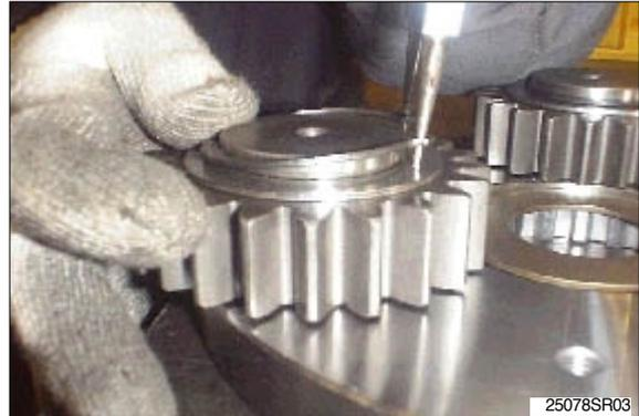
Dismantle needle cage(20) and No.1 side plate(21).
