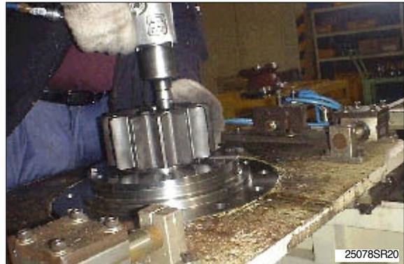
To lock the bolts(28), bend the lock
