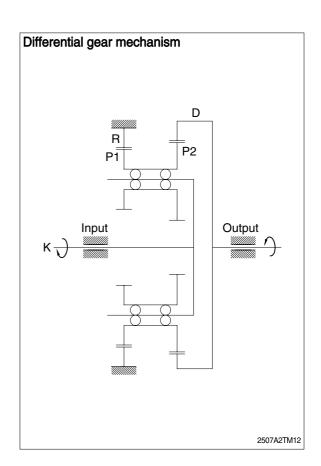
Upon rotation of the sun gear(S) via the input shaft, planetary motion is given among the gears(S), (P1) and (R) and rotation of the gear(P1) around another gear causes the carrier(K) to rotate.
