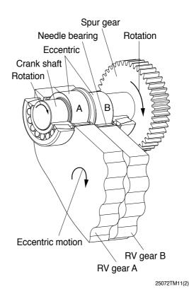
RV gears(4), (5) are fitted up the eccentric crank shaft(9) through bearings. According to rotating of the crank shafts(9), RV gears(4), (5) revolve (Eccentric motion) along pin-gears(17) within hub(1). As these crank shafts are supported by spindle(2), hub (1) rotates with reducing the speed. Gear ratio of second reduction is described as the following.
