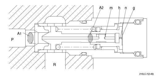
When hydraulic oil pressure( $P \times A_1$ ) reaches the preset force(FSP) of spring(4), the plunger(3) moves to the right as shown.
