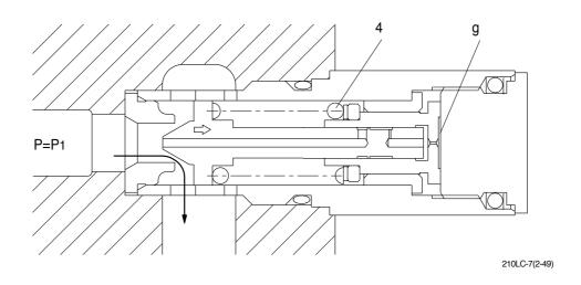
The oil flow chamber g via orifice m and n. When the pressure of chamber g reaches the preset force(FSP) of spring(4), the piston(6) moves left and stop the piston(6) hits the bottom of bushing(7).
