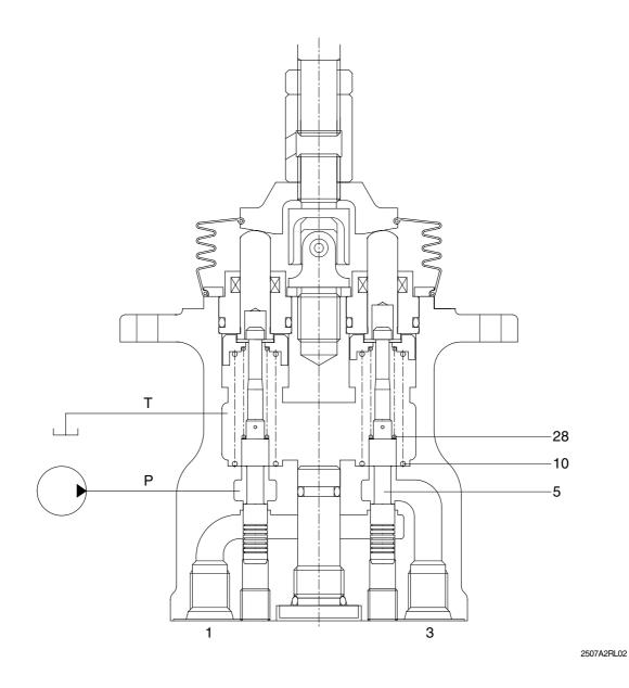
The force of the spring(28) that determines the output pressure of the pilot valve is not applied to the spool(5). Therefore, the spool is pushed up by the spring(10) to the position of port(1, 3) in the operation explanation drawing. Then, since the output port is connected to tank port T only, the output port pressure becomes equal to tank pressure.
