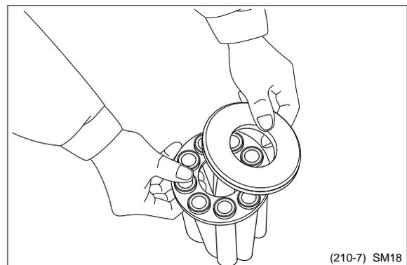
Remove backing spring(4) from cylinder (24).
