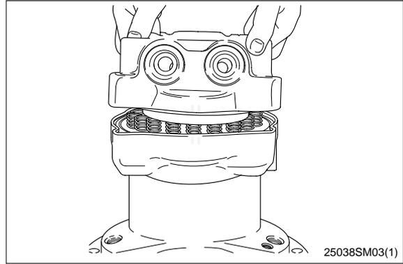
**(17) Tighten cover(33) and housing(25) with 16mm hexagonal socket bolt(36).**
