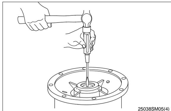
**(17) Disassembly of cylinder assembly**
