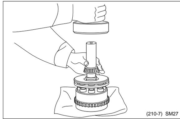
Apply loctite to bearing mounting area of inner race of cylinder(24) lightly.
