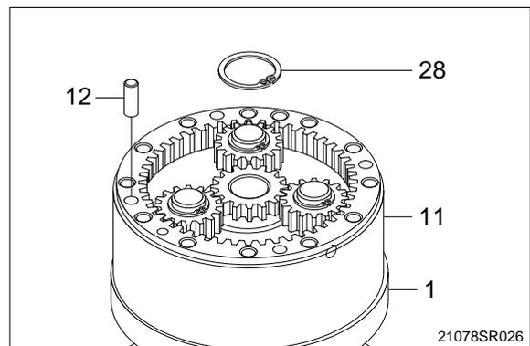
(14) Apply loctite to the tapped holes of the ring gear(11) and then mount swing motor onto the ring gear(11).
