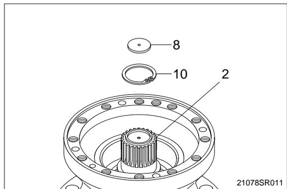
(12) Remove drive shaft(2) with roller bearing(7) and oil seal(6) assembled.
