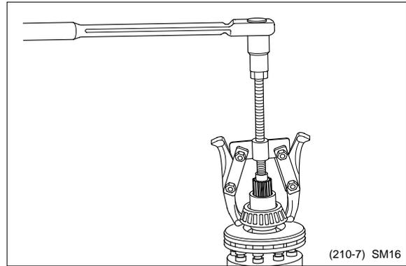
Separate cam plate(5), piston assembly (7), return plate(6) from cylinder(24).
