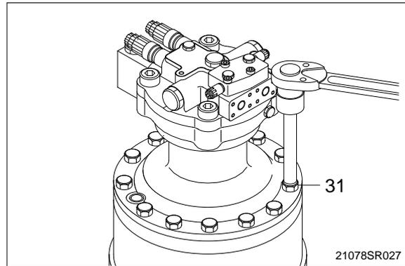
(16) Assemble plugs(29, 30), gauge bar(33) and gauge pipe(32).
