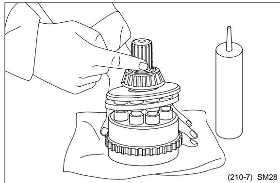
Assemble inner race(1) to cylinder(24).
