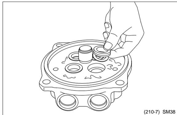
(11) Lubricate locating pin for antirotation of balance plate(21) of cover(33) with grease sufficiently and install locating pin to housing.
