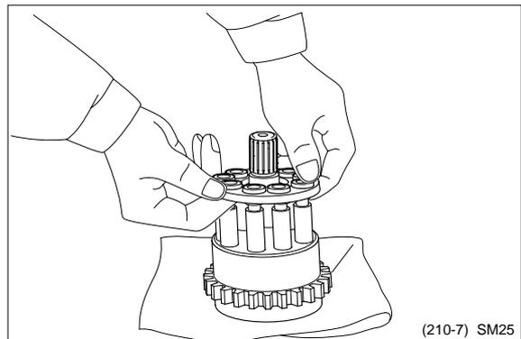
Lubricate specified hydraulic oil on shoe sliding face of piston assembly(7) and assemble cam plate(5).
