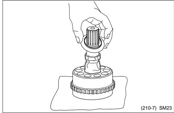
Insert piston assembly(7) in hole of return plate(6).
