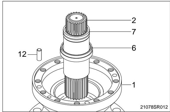
(13) Remove roller bearing(7) and oil seal(6) from the drive shaft(2).
