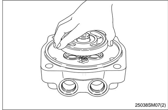
(13) Assemble inner race of needle bearing (22) and snap ring(23) to cover(33).
