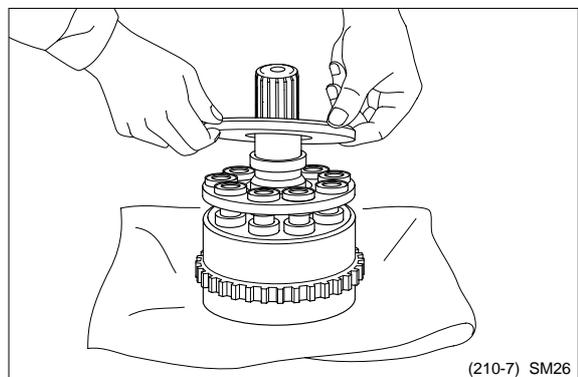
Assemble inner race of taper roller bearing(3) to cylinder(24).
