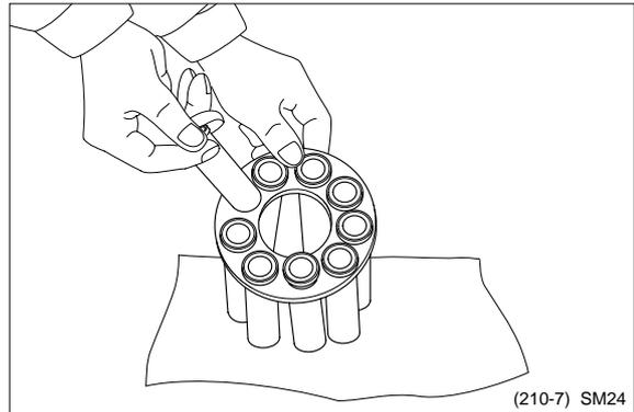
Assemble piston assembly(7) and return plate(6) to cylinder(24). When assembling, check matching mark between them. Before assembling, lubricate specified hydraulic oil in piston hole of cylinder(24).
