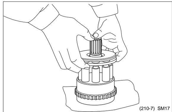
Get cam plate(5) slide on sliding face of piston assembly(7) and remove it. Be cautious not to damage on sliding face of cam plate.
