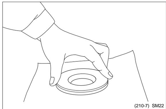
When assembling, lubricate with specified clean hydraulic oil.
