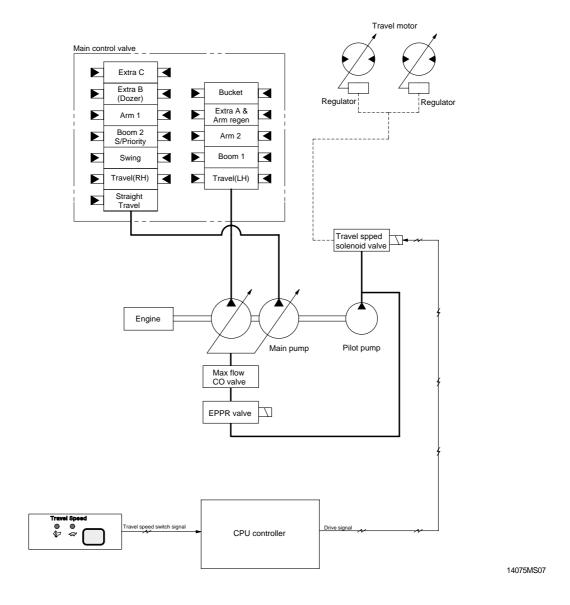
Travel speed can be switched manually by pressing the travel speed switch on the cluster.
