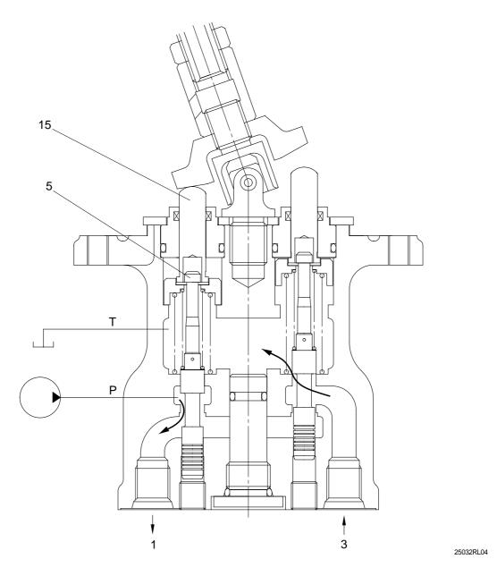
When the push rod(14) is stroked, the spool(5) moves downwards.
