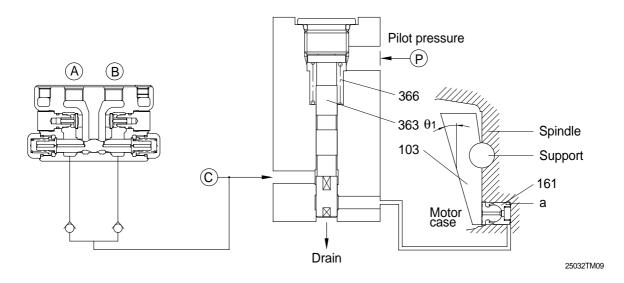
When the pilot pressure is shut off from port , valve(363) is pressed upward by the force of spring(366), the pressurized oil supply port is shut off, and oil in chamber is released into the motor case through the valve(363). Consequently, swash plate(103) is tilted at a maximum angle(1) and the piston displacement of hydraulic motor becomes maximum, thus leading to low-speed operation.
