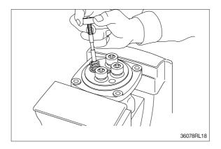
(5) Assemble O-ring (15) onto plug (14).
