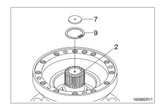
(12) Remove drive shaft (2) with roller bearing(6) and oil seal (5) assembled.Remove knock pin (11) from the casing (1).
