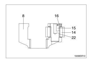
(5) Assemble carrier 2 (8) assembly correctly to the drive shaft (2).
