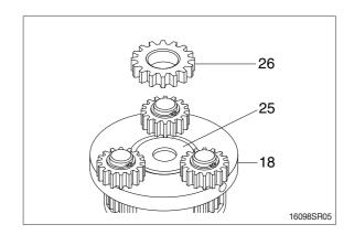
(6) Tighten two M10 eye bolts to carrier 1 (18) and lift up and remove carrier 1 (18) as subassembly.
