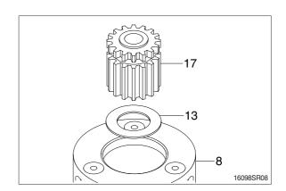
(9) Remove carrier 2 (8) assembly from casing (1).
