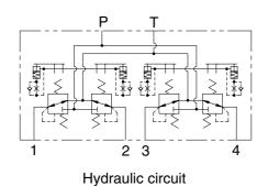
Port Port Port size Ρ Pilot oil inlet port Τ Pilot oil return port 1 Travel (LH, Forward) PF 1/4 2 Travel (LH, Backward) 3 Travel (RH, Forward) 4 Travel (RH, Backward)
