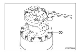
(4) Tighten 3 M16 eye bolts to the ring gear (10) and then lift the ring gear (10) out of the casing (1).
