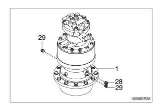
(16) Turn the swing motor assembly upside down and assemble cover plate (33) by tightening the hexagon bolts (34).
