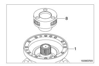
(6) Assemble sun gear 2 (17) and thrust washer (13) to the center of the carrier 2(8) assembly.
