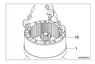
(5) Remove sun gear1 (26) from side plate 3 (25).
