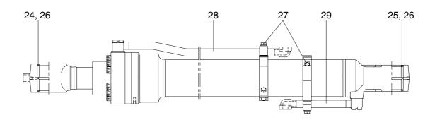
Hexagon socket head bolt 1 Tube assembly 12 Back up ring 23 2 Rod assembly 13 Cushion ring 24 Pin bushing 3 Gland 14 Piston Pin bushing 25 4 DD2 bushing 15 Piston seal 26 Dust seal 5 Snap ring 16 Wear ring 27 Band assembly 6 Rod seal Pipe assembly-R 17 Dust ring 28 7 Back up ring 18 O-ring 29 Pipe assembly-B 8 Buffer ring 19 Back up ring 30 O-ring 9 **Dust wiper** 20 Lock nut 31 Hexagon socket head bolt
