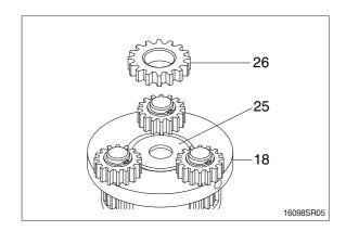
(9) Assemble carrier 1 (18) assembly onto the carrier 2 (8) assembly.
