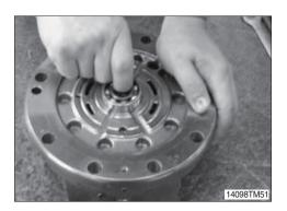
⑥ Install parallel pin (41) into the pin hole of rear flange (1).
