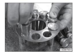
③ Thrust ball (8) from the removed cylinder block (4).
