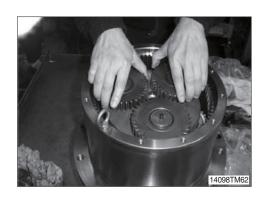
(5) Remove sun gear (114), screw (110) and thrust plate F (113).
