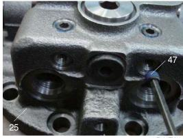
(16) Disassemble plug (37) from valve casing (25) using a torque wrench and disassemble two speed control spool (35), spring (36) in regular sequence.
