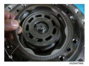
(9) Assemble parking piston (20) into shaft casing (1) using a jig.
