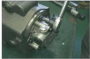
(8) Loosen hexagon socket head bolt (401) which tighten pump casing (271, 272) and valve block (312).
