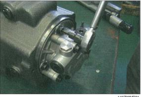
(11) Attach the PTO unit (05) by fastening the flange socket (435) to the valve block (312).
