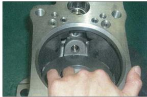
(4) To pump casing (271, 272), fit drive shaft (111, 113) set with bearing (123), bearing spacer (127) and stop ring (824).
