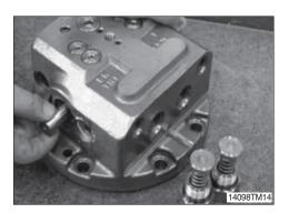
⑤ Install O-ring (37) on the plug (24). Apply grease to the O-ring (37).
