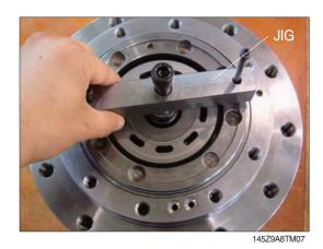
(6) Disassemble friction plate (19)-3EA, steel plate (18)-4EA.
