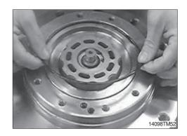
③ Install parallel pins (42, 2EA) into the spindle (101).
