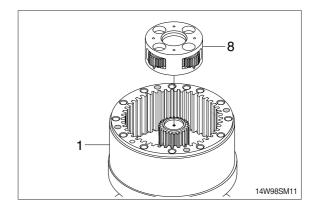
(8) Assemble sun gear 2 (11) and side plate 1 (20) to the center of the carrier 2 (8) assembly.
