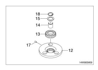
(10) Assemble carrier 1 (12) assembly into the ring gear (21).
