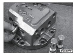
⑥ Install O-ring (37) on the plug (24). Apply grease to the O-ring (37).
