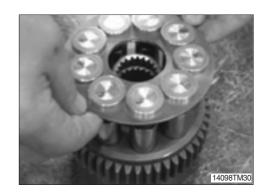
② Piston (5) and shoe (6) from the removed retainer plate (7).
