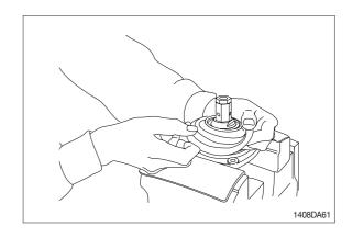
(6) Loosen adjusting nut (21) and swash plate (20) with spanners on them respectively, and remove them.
