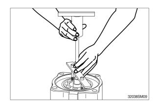
(10) Remove the cylinder (9) from the drive shaft (5) with the motor positioned horizontally. Remove ball guide (11), set plate (12), piston (13) and shoe plate (8).
