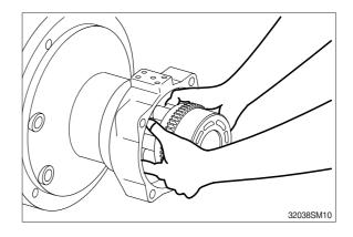
(11) Remove friction plate (14) and separate plate (15) from body (1).
