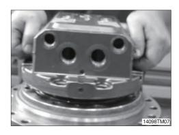
(5) Remove the parallel pin (42) from the spindle (101).
