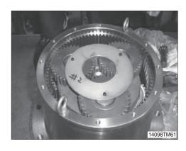
(4) Remove planetary gear R (117), needle bearing, inner race (119) and holder (116) from hub (105).
