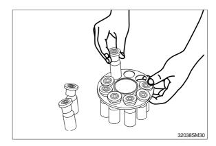
(8) Reassemble the piston assembly (9) to the body (1).
