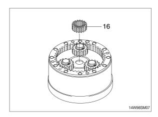
(4) Tighten two M10 eye bolts to carrier 1 (12) and lift up and remove carrier 1 (12) as subassembly.
