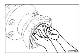
(12) Remove snap ring (4) and remove drive shaft (5) from body (1).
