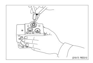
compensating piston (621) and piston case (622) into compensating hole. Fit pilot cover (641) and tighten it with hexagonal socket head screws (436, 438).
