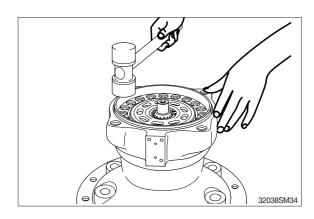
(12) Reassemble brake spring (19) to the brake piston (16).
