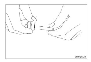
(15) Remove O-ring (15) and seal (16) from plug (14).
