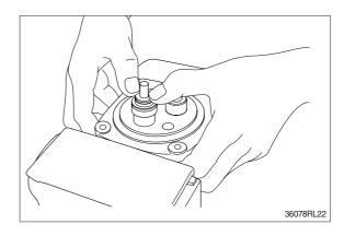
(9) When return spring is strong in force, assemble 4 sets at the same time, utilizing plate (17), and tighten joint (19) temporarily.
