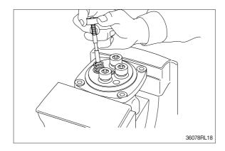
(5) Assemble O-ring (15) onto plug (14).
