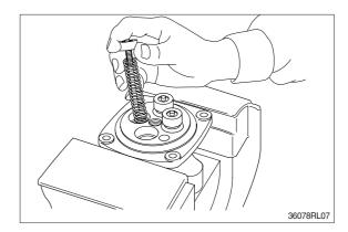
(11) Loosen hexagon socket head plug(2) with hexagon socket screw key.
