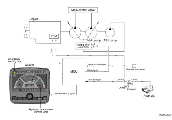
1. If the engine coolant temperature or the hydraulic oil temperature is overheated over 100°C, the warning lamp is ON and the pump input torque or the engine speed is reduced as below logic table.
