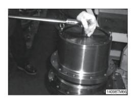
(6) Install thrust washer (109) and collar (112) into the hub (105).
