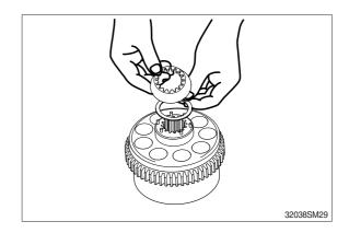
(7) Install the piston sub-assembly (13) to the set plate (12).
