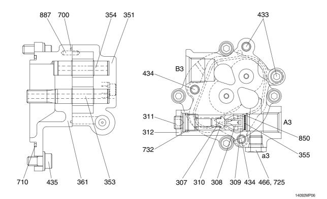
353 Drive gear 307 Poppet 466 Plug 308 Seat 354 Driven gear 700 Ring 309 Ring 355 Filter 710 O-ring 310 Spring 361 Front case 725 O-ring 311 Screw 433 Flange socket 732 O-ring 312 Nut 434 Flange socket 850 Snap ring 435 Flange socket 351 Gear case 887 Pin
