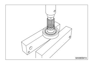
(14) Remove bushing (6) and oil seal (2) from body (1).
