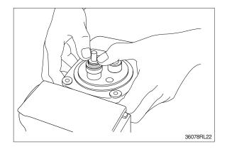
(9) When return spring is strong in force, assemble 4 sets at the same time, utilizing plate (17), and tighten joint (19) temporarily.
