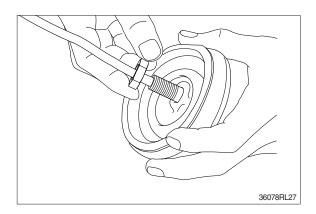
(16) Pull out cord and tube through adjusting nut hole provided in direction 60° to 120° from casing hole.
