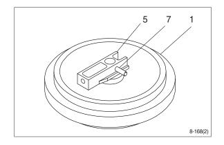
⑧ Lay bracket (5) on its side. Supply engine oil to the specified level, and tighten plug.
