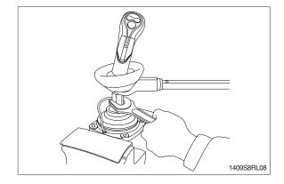
(19) Apply grease to rotating section of joint and contacting faces of disk and push rod.
