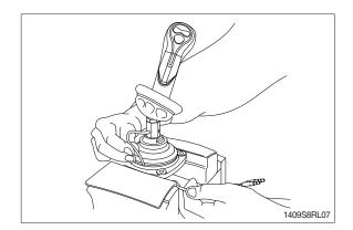
(18) Determine handle direction, tighten lock nut (22) to specified torque to fix handle.
