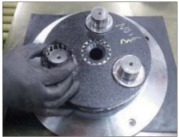
3) Assemble planetary gear No.1 (14) of which groove is faced downward. (3 places)
