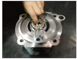
(27) Apply grease on steel side of valve plate (20) to prevent plate from sliding.
