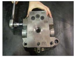
(9) Remove plug (29) (1EA), plug (27) (2EA) using 4 mm, 6 mm hexagon wrench.
