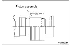
6 Fit piston nut (23) and tighten the set screw (24).
