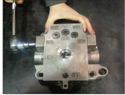
(23) Caulk check valve (23) using jig. (same for the set on opposite side)
