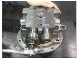
(5) Unscrew socket bolt (42) (4EA) using 12 mm hexagon wrench.
