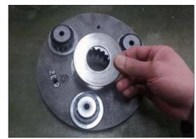
(7) Assemble planetary gear No.1 (18) of which groove is faced downward.(3 pcs)
