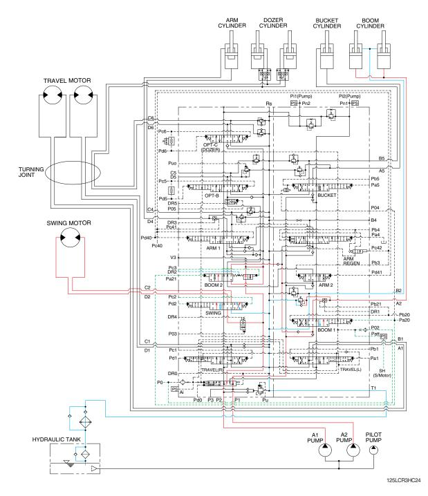
When the swing and boom up functions are operated, simultaneously the swing spool and boom spools in the main control valve are moved to the functional position by the pilot oil pressure from the remote control valve.
