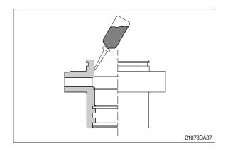
② Coat dust wiper (11) with grease and fit dust wiper (11) to the bottom of the hole of dust seal.
