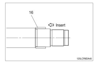
(5) Fit piston assembly to rod assembly. Tightoning t e :
