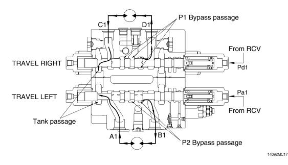
During the travel forward operation, the hydraulic fluid of the pump A2 is supplied to the travel left motor and the hydraulic fluid of the pump A1 is supplied to the other travel right motor.
