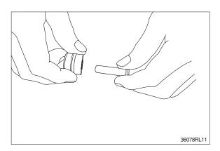
(15) Remove O-ring (15) and rod seal (16) from plug (14).
