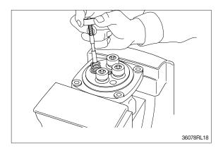
(5) Assemble O-ring (15) onto plug (14).
