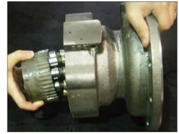
(11) Put friction plate (13) in casing.
