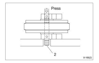
6 Remove the bushing (4) from idler, using a special tool.
