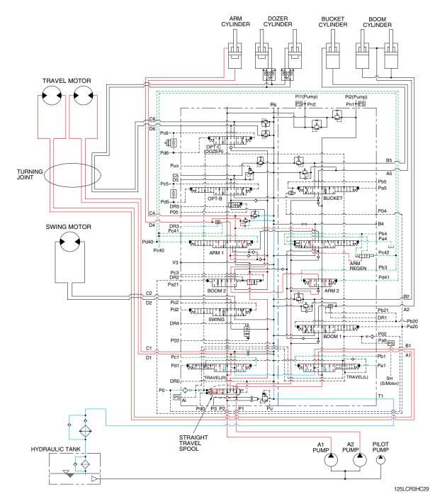
When the arm and travel functions are operated, simultaneously the arm spools and travel spools in the main control valve are moved to the functional position by the pilot oil pressure from the remote control valve and the straight travel spool is pushed to the right by the oil pressure from pilot pump. The oil from the A1 pump flows into the travel motors through the RH travel spool of the left control valve and the LH travel spool of the right control valve via the straight travel spool.
