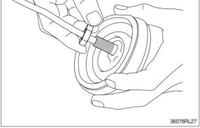
(14) Pull out cord and tube through adjusting nut hole provided in direction 60 °to 120 °from casing hole.
