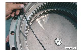
(41) By using a tackle and the equipment place the end cover (4) on the toothed ring (19).
