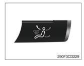
① Operating this switch, it beeps and displays symbol of each mode in order. (Face  $\rightarrow$  Face/Rear  $\rightarrow$  Face/Rear/Foot  $\rightarrow$  Foot  $\rightarrow$  Def/Foot)
