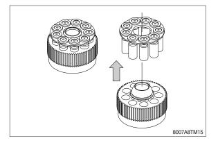
b. Remove piston assy (6) from retainer plate (7).
