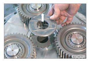
(13) By using a tackle and the equipment remove the 1st reduction assembly (8).
