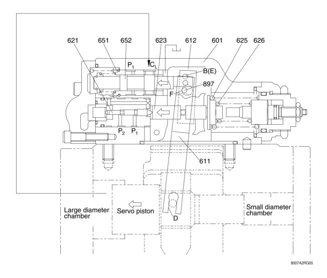
As the self pump delivery pressure P1 or the companion pump delivery pressure P2 decreases, the compensating rod (623) is pushed back by the action of the springs (625 & 626) to rotate lever 1 (612) around point E. Rotating of lever 1 causes the feedback lever (611) to rotate around the fulcrum of point D and then the spool (652) to move to the left. As a result, port CL opens a way to the tank port.
