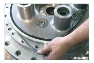
(27) By using a rubber hammer push the 6 pins (20) against the shoulder until assembly is completed.
