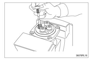
(3) Assemble O-ring (10) onto plug (8).
