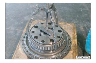
(36) Remove the spacer (24) from its seat in the flanged hub (27).
