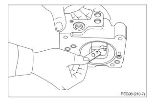
(10) Draw out pin (874) and remove feedback lever (611).
