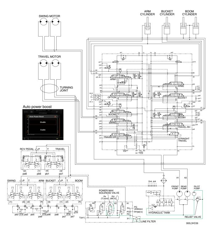
When the power max switch on the left control lever is pushed ON, the power max solenoid valve is actuated, the discharged oil from the pilot pump flow into PH port of the main relief valve of main control valve ; Then the setting pressure of the main control valve is raises from 330 kgf/cm<sup>2</sup> (4690 psi) to 360 kgf/cm<sup>2</sup> (5120 psi) for increasing the digging power. And even when press continuously, it is canceled after 8 seconds.
