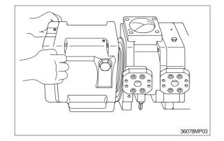
(11) Tapping lightly fitting flange section of swash plate support (251) on its pump casing side, separate swash plate support from pump casing.
