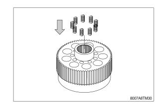
⑧ Install retainer holder (8) on cylinder block (4).
