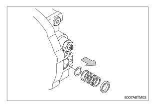
② Remove spool assy (2-2) turning slowly. Be careful not to damage around the spool assy.
