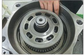
\* At first, insert a separator plate (743), and then insert a friction plate (742) and separator plate alternately.
