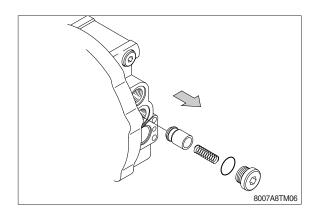
⑤ Remove Plugs (2-14, 2-17) remove spring (2-13) and spool assy (2-9).
