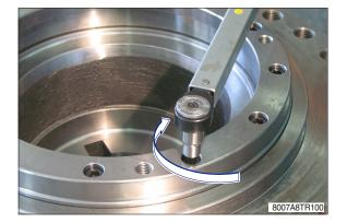
\* Before assembling the hydraulic motor, verify by a depth slide gauge the correct assembly of the unit checking the axial distance as shown in the figure.
