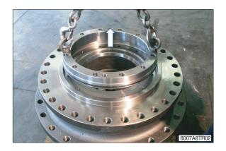
(3) Remove the O-ring (28) from its seat in the motor adapter (29).
