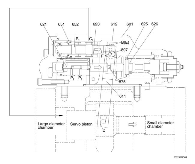
When the self pump delivery pressure P1 or the companion pump delivery pressure P2 rises, it acts on the stepped part of the compensating piston (621). It presses the compensating rod (623) to the right till the force of the outer spring (625) and inner spring (626) balances with the hydraulic force. The movement of the compensating rod is transmitted to lever 1 (612) via pin (875).
