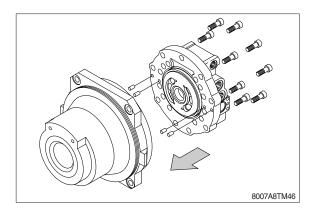
Place spring (2-13) on valve assy (2-9), and then install valve assy on base plate (2-1).
