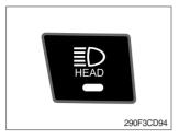
This switch is used to operate the head light.
