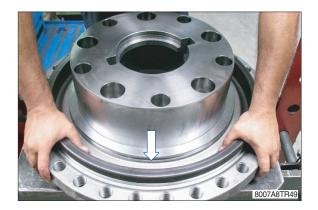
(7) Assemble the bearing inner ring (21) in the flanged hub (27).
