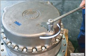
(7) Unscrew the 21 socket head screws (1) from the end cover (4).
