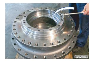
(2) By using a tackle remove the motor adapter (29).
