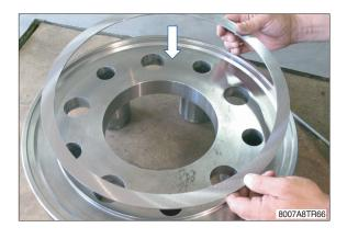
(21)By using a rubber hammer push the spacer (18) against the shoulder until assembly is completed.
