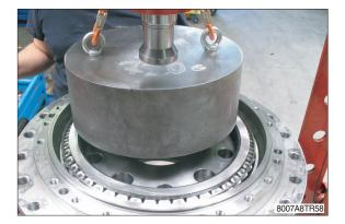
(15) By using a press and the stopper push the bearing inner ring (21) against the shoulder of the flanged hub (27) until assembling of the unit is complete.
