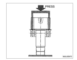
(14) Remove oil seal (801) from casing (102)
