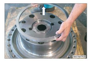
(37) By using pliers remove the circlip (25) from its seat in the flanged hub (27).
