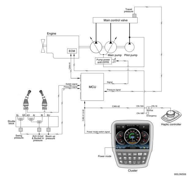
• The variable power control system controls the engine and pump mutual power according to RCV lever stroke and pump load.
