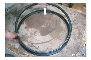
(6) Assemble the 1st half seal (23) in the flanged hub (27).
