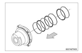
Apply grease to O-rings (22)(24), backup ring (23)(25), and install them to brake piston (21).
