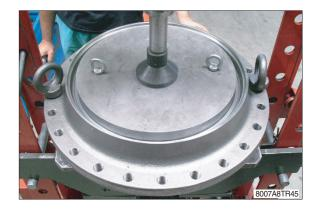
(4) Insert the spacer (24) on the flanged hub (27).
