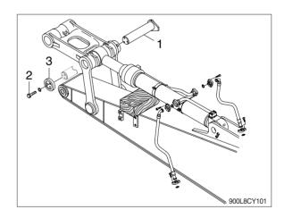
③ Disconnect bucket cylinder hoses (4) and put plugs (5) on cylinder pipe.
