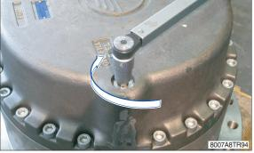
(45) Assemble the O-ring (28) into its seat in the motor adapter flange (29).
