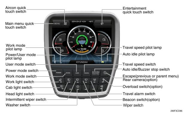
When some of the switches are selected, the pilot lamps are displayed on the LCD. Refer to the page 5-91 for details.
