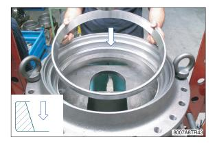
(2) Place the equipment on the bearing outer ring (21).
