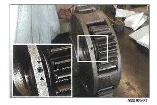
(10) Apply liquid packing to casing (102).
