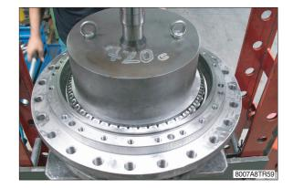
(16) By using a tackle remove the gearbox by the press.
