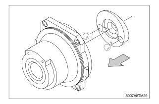
⑦ Install 9 springs (17) on cylinder block (4).
