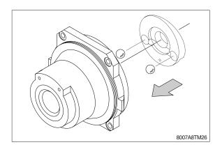
⑤ Press fit Inner race of roller bearing (13) on shaft (3).And then, install shaft sub assy on case
