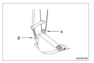
② Remove bolt (1), stopper (2) and draw out the pin (A).
