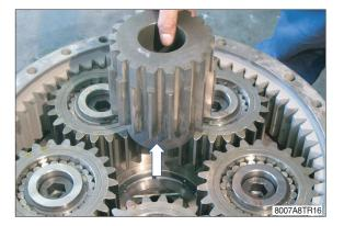
(17) By using a crowbar lift the toothed ring (19) from the gearbox housing (22).
