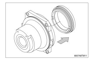
\* Before work, put rag on all surface of brake piston because brake piston fly out and oil flies off while at work.
