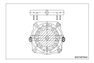
Install springs (26) in the holes of brake piston (21).
