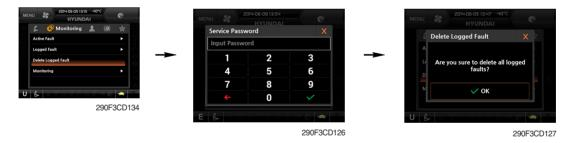
• The logged faults of the MCU, engine ECM or air conditioner can be deleted by this menu.
