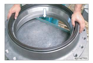
X Correct lifetime seal (23) assembly check.
