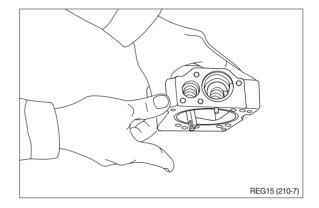
(13) Install cover (C, 629) fitted with adjusting screws (628, 925), adjusting ring (C, 627), lock nut (630), hexagon nut (801) and adjusting screw (924).
