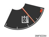
① This gauge indicates the temperature of hydraulic oil.
