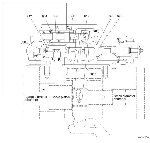
The set horsepower valve is shifted by varying the command current level of the proportional pressure reducing valve attached to the pump. Only one proportional pressure reducing valve is provided. However, the secondary pressure Pf (power shift pressure) is admitted to the horsepower control section of each pump regulator through the pump's internal path to shift it to the same set horsepower level.
