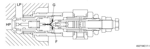
(3) When above flow is formed, the pilot poppet is opened; the pressure of chamber (D) drops, the main poppet (C) is opened and then the oil directly flows into the low pressure passage (LP).
