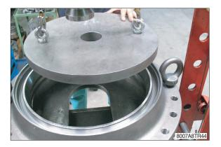
(3) By using a press and the stopper push the bearing outer ring (21) against the gearbox housing shoulder (22).
