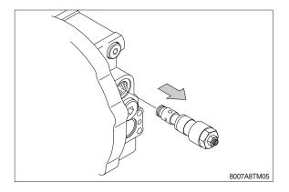
④ Remove plug (2-21), spring (2-20) and check valve (2-19).
