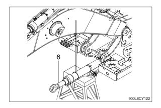
(5) Disconnect boom cylinder hoses (7) and put plugs on cylinder pipe.
