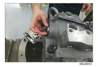
(8) Remove socket head bolts (401) and remove valve casing (303) from casing (301) then remove valve plate (131).
