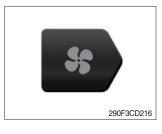
① This switch used to select air conditioner control mode.
