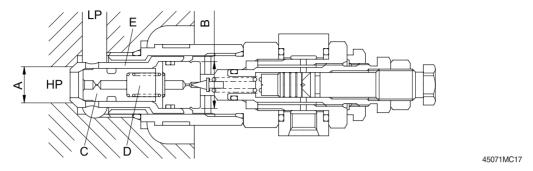
(2) When the pressure in neutral passage (HP) reaches the setting force of spring, pilot poppet (F) is opened.
