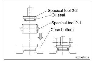
② Press fit the outer race of roller bearing (13) in case (1).
