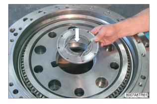
(18) By using a rubber hammer push the discs retainer (26) against the shoulder until assembly is complete.
