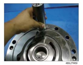
(8) Apply loctitle #242 on the restrictor (57, 58) and then assemble restrictor (57, 58), O-ring (43, 44) into rear cover (34).
