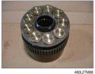
(21) Assemble cylinder block kit into casing (1).
