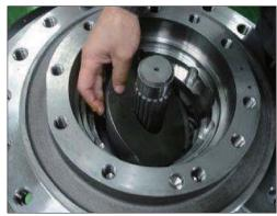
(10) Disassemble steel ball (13), swash piston (6) Hole in the casing (1) of two speed line is decomposed by injecting oil.
