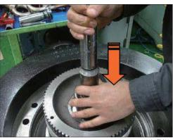
(14) Disassemble valve plate (28) into rear cover (32).
