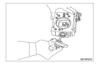
(5) After removing cover (C, 629) subassembly, take out outer spring (625), inner spring (626) and spring seat (C, 624) from compensating section.
