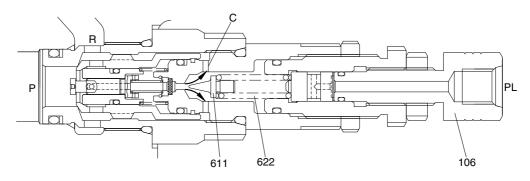
③ Opening of the poppet (611) causes the pressure in chamber B to fall and the plunger (511) to open. As the result the pressurized oil in the path (P) runs into the low pressure path (R) directly.
