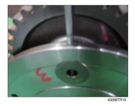
⑤ Caulking both side of pressed spring pin 180° using caulking jig.
