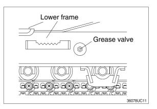
(2) Jack up the track link height enough to permit carrier roller removal.
