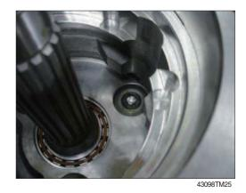
(11) Disassemble pivot (14, 2EA) from casing (1).
