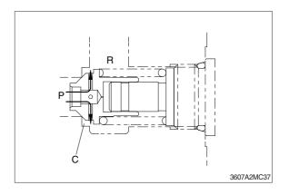
③ When the pressure in the path (P) goes over the set pressure of the spring (621), the poppet (611) opens. Then, the pressurized oil in the path (P) passes around the outside of the poppet (611) and flows to the low-pressure path (R). P 611 3607A2MC38
