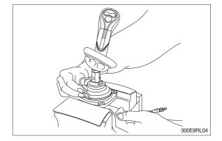
(16) Determine handle direction, tighten lock nut (22) to specified torque to fix handle.
