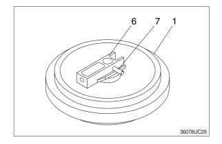
⑧ Lay bracket (6) on its side. Supply engine oil to the specified level, and tighten plug.
