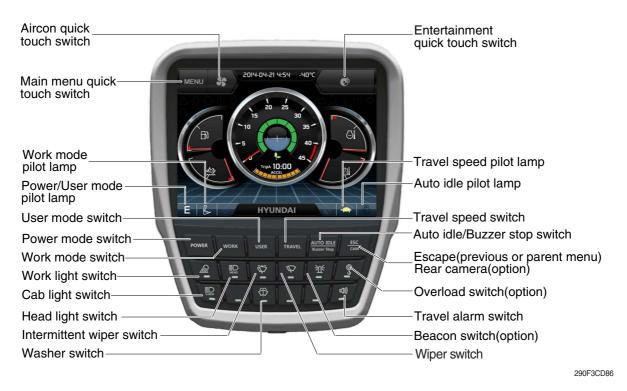
When some of the switches are selected, the pilot lamps are displayed on the LCD. Refer to the page 5-71 for details.
