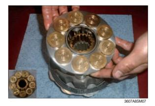
② Disassemble ball guide (12), friction plate (15), plate (16) and ball guide seat (11) from cylinder block (9).
