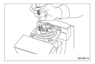
(3) Assemble O-ring (10) onto plug (8).
