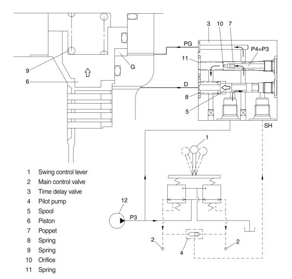
b. When all of the RCV lever (1) are set the neutral position, the spool (5) returns to right.
