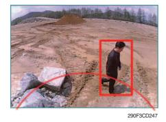
· When the worker or pedestrian go to the blue line (radius 5 m), an external danger area of equipping on the cluster screen, the warning buzzer sounds and it displays the blue rectangular box for the recognition of the worker and pedestrian.
