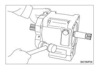
(12) Remove shoe plate (211) and swash plate (212) from pump casing (271).
