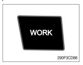
① This switch is to select the machine work mode, which shifts from general operation mode to optional attachment operation mode.
