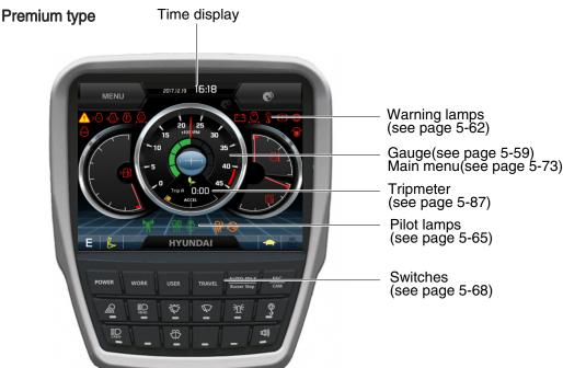
\* The warning lamp pops up and/or blinks and the buzzer sounds when the machine has a problem. The warning lamp blinks until the problem is cleared. Refer to page 5-62 for details.
