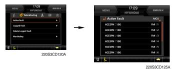
· The active faults of the MCU can be checked by this menu.
