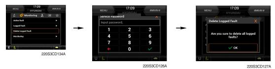
· The logged faults of the MCU can be deleted by this menu.
