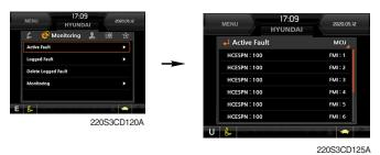
· The active faults of the MCU can be checked by this menu.
