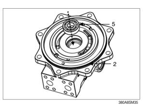
(18) Apply some grease to the back side of the valve plate (18) and align the hole of the pin (22) and assemble it on the valve casing (2).
