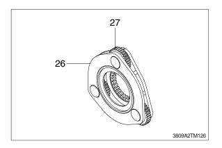
(16)Remove planetary gear C (27) from No.3 carrier C (26).
