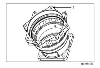
(3) Assemble the oil seal (6) on the casting (1).
