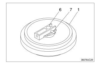
8 Lay bracket (6) on its side.Supply engine oil to the specified level, and tighten plug.
