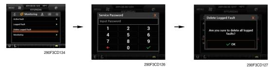
The logged faults of the MCU, engine ECM, air conditioner or AAVM can be deleted by this menu.
