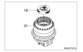
(18) Assemble plate (36) to carrier B (18).
