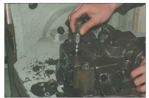
③ Remove plug (564) from valve casing (303). And then screw two  $M10 \times 135$ bolts on the holes of compelling brake release. Sub assembly (valve casing & brake piston)
