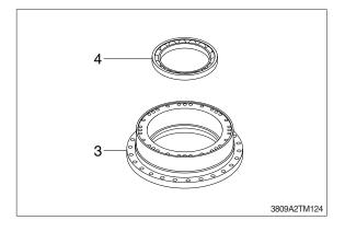
(15)Remove floating seal (2) and angular bearing (4) at opposite of hub (3).
