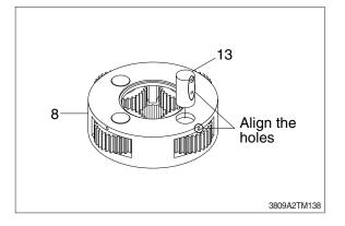
④ Assemble carrier (8) and pin (13) striking pin (14) by hammer.
