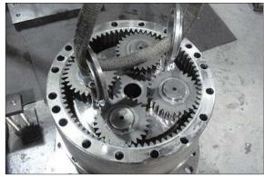
② Insert sun gear 1 (27) to planetary gear 1 (18).
