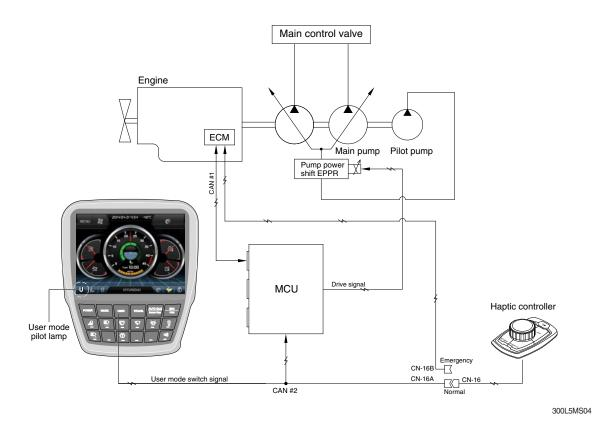
1) High idle rpm, auto idle rpm and EPPR pressure can be adjusted and memorized in the U-mode.
