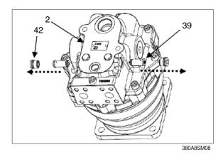
(6) Remove the RO plug (42) from the valve casing (2) and pull out the reactionless valve (39).
