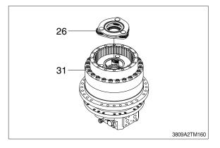
(21)Assemble carrier C (26) to drive gear (34).
