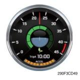
(3) Engine coolant temperature gauge
