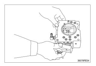
(7) Remove snap ring (814) and take out spring seat (653), return spring (654) and sleeve (651).
