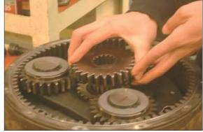
(6) Remove carrier 1 (5), together with planetary gears 1 (12), sun gear 2 (10), etc. fitted.
