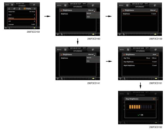
If "Auto" is chosen, brightness for day and night can be differently set up. Also by using the bar in lower side, users can define which time interval belongs to day and night. (in bar figure, white area represents night time while orange shows day time)
