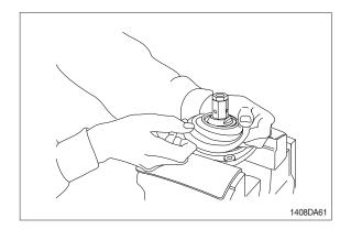
(6) Loosen adjusting nut (17) and swash plate (16) with spanners on them respectively, and remove them.
