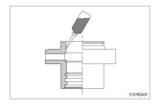
② Coat dust wiper (9) with grease and fit dust wiper (9) to the bottom of the hole of dust seal.
