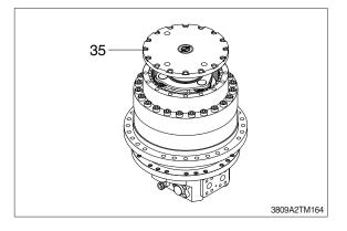
(25)Assemble cover (35) and tighten them to the specified torque.
