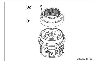
(13)Remove hub (3) from assembly (1). - Tools : I-bolt, Hoist
