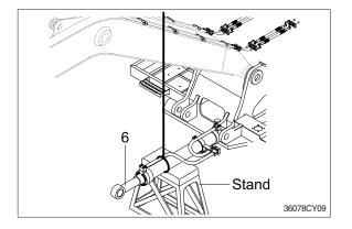
⑤ Disconnect boom cylinder hoses (7), and put plugs on cylinder pipe.
