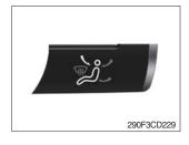
Operating this switch, it beeps and displays symbol of each mode in order. (Face → Face/Rear → Face/Rear/Foot → Foot → Def/Foot)
