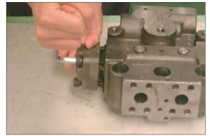
⑦ Assemble tilting spool (531), tilting spring (533) and plug (571) in the order named.  $\cdot$  Tightening torque : 7.5 kgf  $\cdot$  m (54.2 lbf  $\cdot$  ft)
