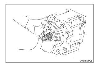
(11) Tapping lightly fitting flange section of swash plate support (251) on its pump casing side, separate swash plate support from pump casing.
