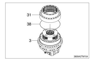
(14) Tighten hub and ring gear.
