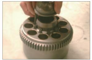
② Put piston (121), shoe (122) subassembly in set plate (123) and then assemble them to cylinder block (111).
