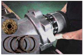
⑤ Disassemble shoe plate (8) from body (1).
