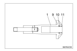
7 Remove rod packing (9), back up ring (10) and dust seal (11).
