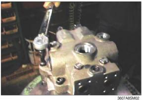
6 Assemble time delay valve assy (31) into rear cover (23) with a wrench bolt (32).
