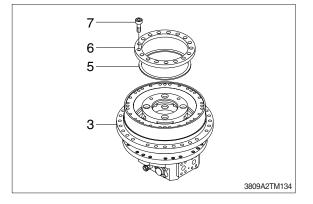
(6) Assemble bearing guide.According to the hub turn, we can check it goes on smoothly or not.
