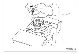
(3) Assemble O-ring (10) onto plug (8).
