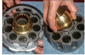
③ Disassemble spring (10) from cylinder block (9).
