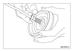
(14) Pull out cord and tube through adjusting nut hole provided in direction 60° to 120° from casing hole.
