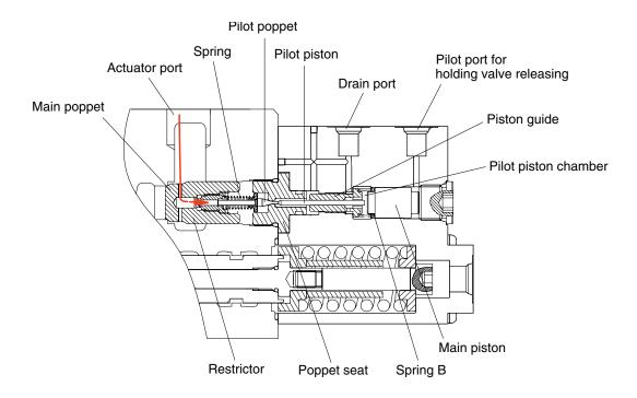
HOLDING VALVE BLOCK SECTION
