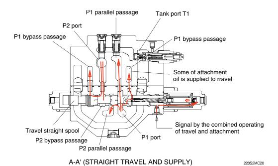
After changeover of the travel straight spool, the pressurized oil discharged from the P1 pump is connected with P2 port oil and is supplied to the attachment line through both parallel passage of the P1 and P2.
