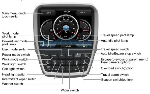
When some of the switches are selected, the pilot lamps are displayed on the LCD. Refer to page 5-65for details.
