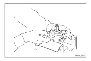
(6) Loosen adjusting nut (17) and swash plate (16) with spanners on them respectively, and remove them.
