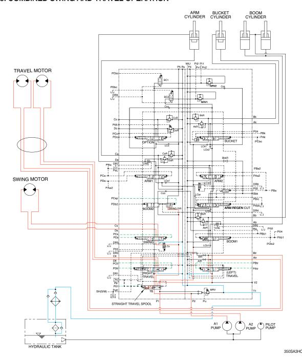
When the swing and travel functions are operated, simultaneously the swing spool and travel spools in the main control valve are moved to the functional position by the pilot oil pressure (PCs, PDs, PAtr, PBtr, PCtl, PDtl) from the remote control valve and straight travel spool is pushed to the right by the pilot oil pressure from the pilot pump.
