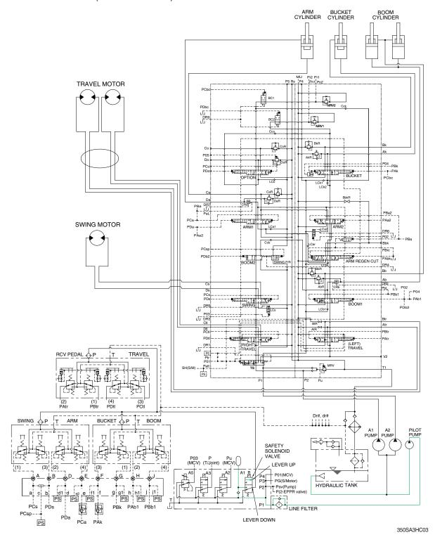
When the lever of the safety solenoid valve is moved upward, oil flows into the remote control valve through solenoid valve and line filter.
