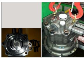
① Assemble level gauge (36) and plug (39) into casing (1).
