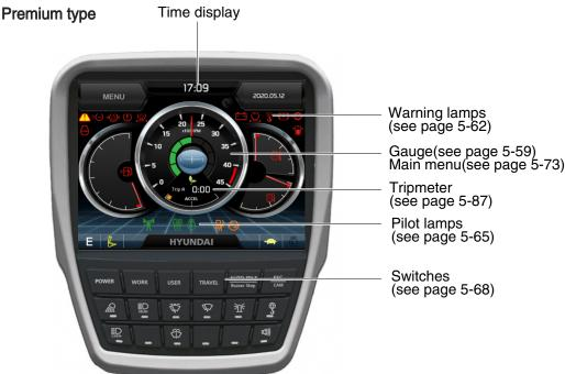
\* The warning lamp pops up and/or blinks and the buzzer sounds when the machine has a problem. The warning lamp blinks until the problem is cleared. Refer to page 3-62 for details.
