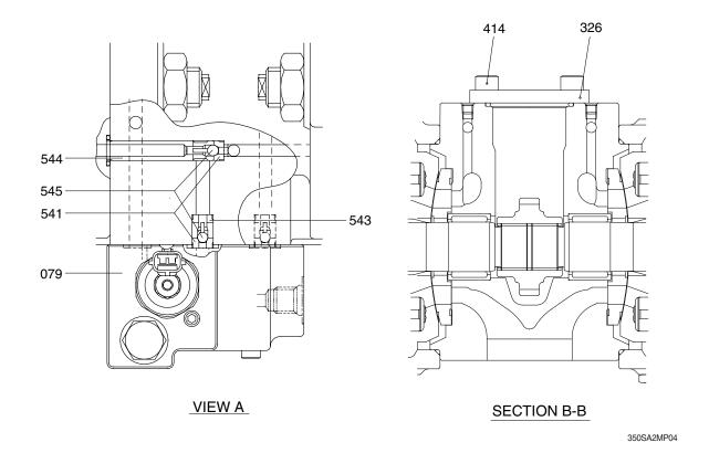
079Proportional reducing valve541Seat544Stopper 2326Cover543Stopper 1545Steel ball
