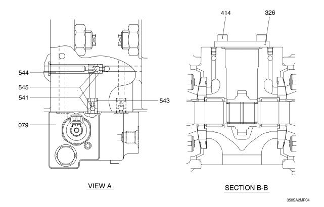
079Proportional reducing valve541Seat544Stopper 2326Cover543Stopper 1545Steel ball
