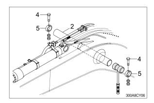
① Lower the boom cylinder assembly (6) on a stand.
