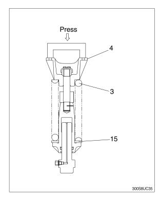
⑥ Lighten the press load and confirm the set length of spring (3).
