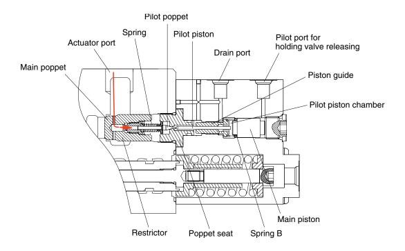
HOLDING VALVE BLOCK SECTION
