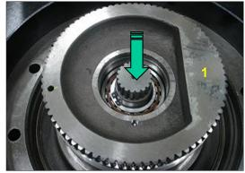
(14) Assemble oil seal(3) into trust block (4) with a assembling jig and press it into casing (1). Caution the direction of oil seal (3).
