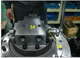
(2) Disassemble wrench bolt (54) using torque wrench.
