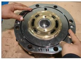
(9) Install casing (1) into assembling jig.
