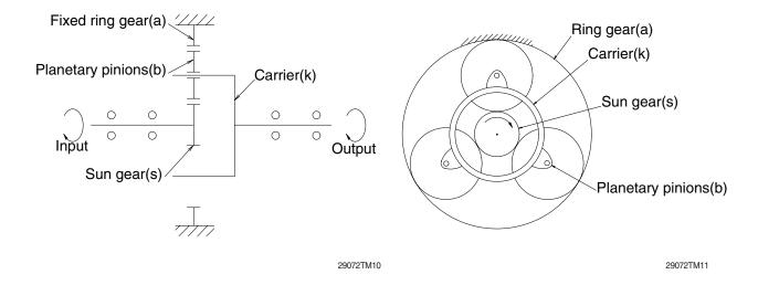
When the sun gear S1 is driven by input shaft, planetary action occurs among gears S1, a and b and revolution of gear b transfers the rotation of carrier K1 to second sun gear S2, and also evokes planetary action between gear S2, a and d.
