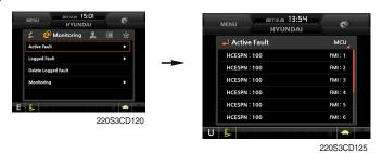
$\cdot\,$  The active faults of the MCU, can be checked by this menu.
