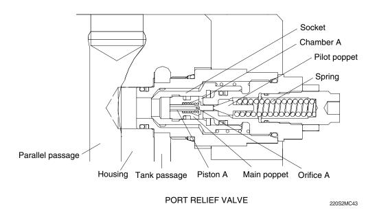
② When the pressurized oil from the actuators becomes equal to the set pressure of the spring, the hydraulic oil apply to the pilot poppet and pushes the pilot poppet to the right direction and flows to tank passage through the piston A internal passage, orifice A, chamber A, periphery orifice B and the hole E.
