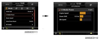
Engine high idle rpm, auto idle rpm and pump torque (power shift) can be modulated and memorized separately in U-mode.
