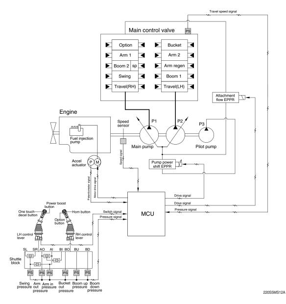
1. When the requirement of pump flow rate is low, IPC mode controls pump flow rate to improve fuel efficiency.
