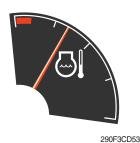
① This gauge indicates the temperature of coolant.
