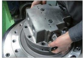
(27) Assemble rear cover (34) into casing (1) and then tighten the wrench bolt (54, 55) using torque wrench.
