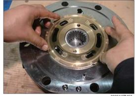
(8) Apply grease to the O-ring and then assemble O-ring into rear cover (34).
