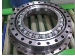
(2) Insert angular bearing (2) into reversed housing (7) on the same way.
