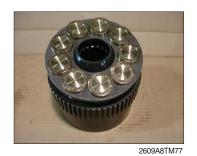
(21) Stant the casing (1) and then assemble cylinder block kit into casing (1).
