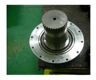
4 After heating sph. roller bearing (3) for 13 minutes at 80~90°C and doing demagnetization, then assemble it to drive shaft (2).
