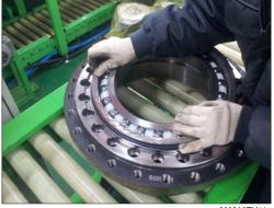
2 Release 25 hex wrench bolts (28. M18) and remove ring gear (1) from housing (7).
