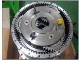
(6) Removing sun gear No.2 Pull away sun gear No.2 (17) for removing.
