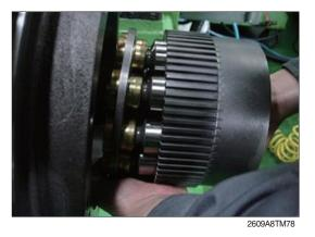
(22) Assemble separated plate (24), friction plate(23) into cylinder block in regular sequence.Friction plate : 4EASeparated plate : 5EA
