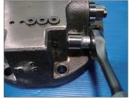
(18) Disassemble plug (58) from rear cover (34).
