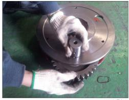
② Then remove planetary gear No.1 (19) and thrust washer No.1 (21) from carrier No.1 (18).
