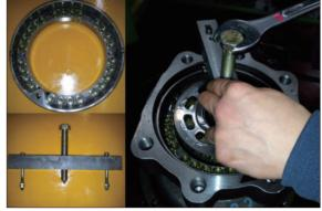
5 Disassemble respectively cylinder block sub (8), friction plate (13), separate plate (14) from casing (1).
