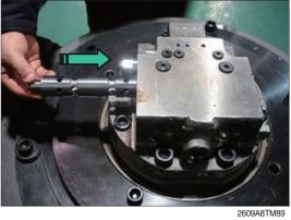
(29) Assemble spring (38), plug (37) into rear cover (34) in regular sequence and then plug (37) into rear cover (34) using torque wrench.
