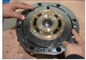
(9) Install casing (1) into assembling jig.
