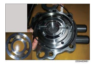
② Using a torque wrench, disassemble relief valve assy (30) from valve casing (23).
