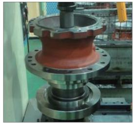
(2) Assemble oil seal to casing.
