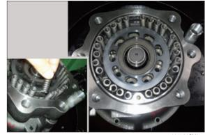
(9) Lift up valve casing (23) on casing (1) by a crane and assemble it with socket bolts (37, 38).
