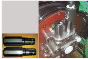
③ Using a torque wrench, disassemble plug (32) from valve casing (23) and disassemble O-ring (33, 34) and reactionless valve assy (31).
