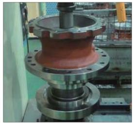
(2) Assemble oil seal to casing.
