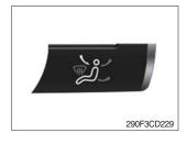
① Operating this switch, it beeps and displays symbol of each mode in order. (Face → Face/Rear → Face/Rear/Foot → Foot → Def/Foot)
