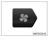
This switch used to select air conditioner control mode.
