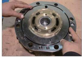
(9) Install casing (1) into assembling jig.
