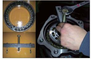
5 Disassemble respectively cylinder block sub (8), friction plate (13), separate plate (14) from casing (1).
