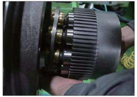
(8) Disassemble cylinder block (18), retainer plate (21), piston assy (22), ball guide (20) and spring (19) into cylinder block kit.
