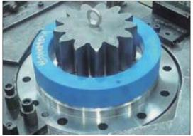
(2) Put drive shaft sub assy into casing.
