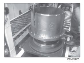
② Setting reduction unit on work stand for disassembling. Remove M16 hexagon socket head bolts that secure ring gear and housing assembly.
