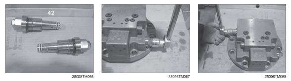
(20) Disassemble both side of the plug (48) and connector (52) from the rear cover (34) by using the torque wrench and then disassemble the spring (51), spring seat (49), parallel pin (50) and spool (47) in order.
