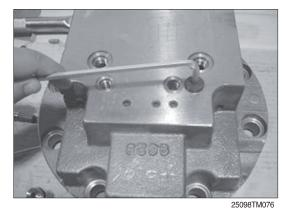
(2) Apply the loctite #242 on the NPTF 1/16 plug (2, 12EA) and tighten it.
