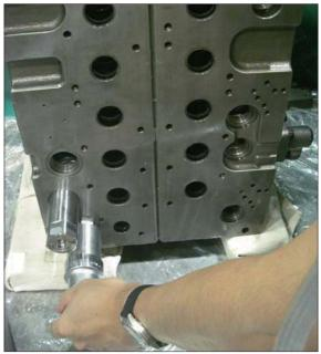
(6) Assembly of arm regeneration cut valve (257) :
