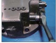
(18) Disassemble plug (57) into rear cover (34).
