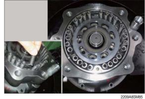
④ Lift up valve casing (23) on casing (1) by a crane and assemble it with socket bolts (37, 38).
