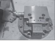
(5) Tight fit the needle bearing (10) into rear cover (34) by using pressing jig.
