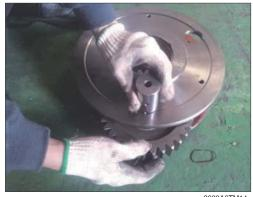
② Then remove planet gear No.1 (19) and thrust washer No.1 (21) from carrier No.1 (18).
