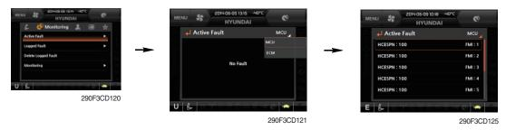
· The active faults of the MCU or engine ECM can be checked by this menu.
