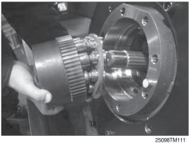
(22) Assemble the separated plate (24) and friction plate (23) into the cylinder block alternately.
