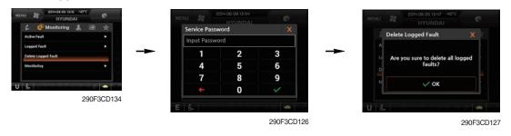
· The logged faults of the MCU or engine ECM can be deleted by this menu.
