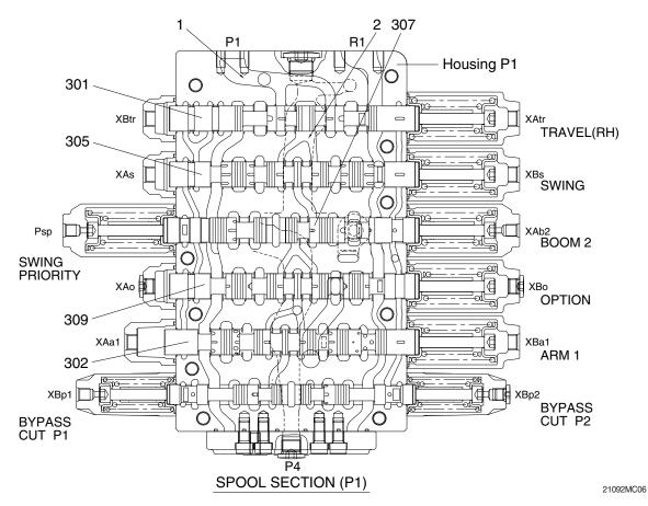
When all spools are in the neutral positions, the pressurized oil discharged from the hydraulic pump (A1) passes through Port P1, the main path (1), the bypass circuit (2) passing the spools for travel right (301), swing (305), boom confluence (boom 2; 307), option (309) and arm 1 (302), and the arm 1 side posi-nega conversion valve (611), and returns to the hydraulic oil tank through the tank port (R1).
