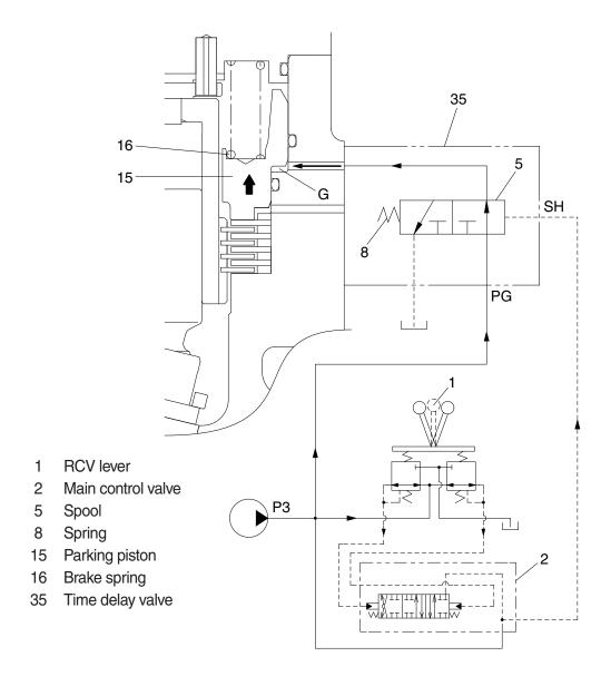
b. When all of the RCV lever (1) are set the neutral position, the spool (5) returns to right.Then, the parking piston (15) is moved lower by spring force and the return oil from the chamber G flows back to tank port.At this time, the brake works.
