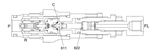
c. Opening of the poppet (611) causes the pressure in chamber B to fall and the plunger (511) to open. As the result the pressurized oil in the path (P) runs into the low pressure path (R) directly.
