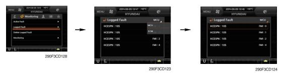
· The logged faults of the MCU or engine ECM can be checked by this menu.
