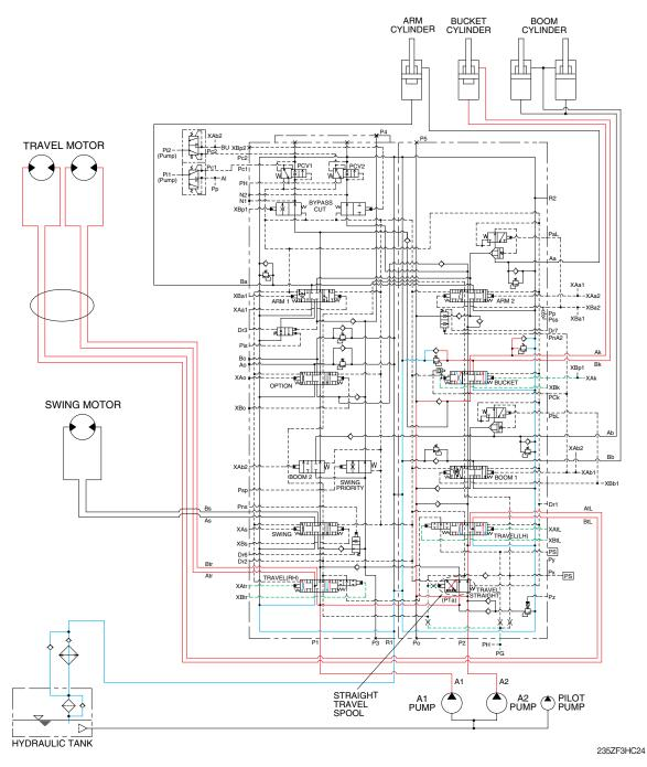
When the bucket and travel functions are operated simultaneously, the bucket spool and travel spools in the main control valve are moved to the functional position by the pilot oil pressure from the remote control valve, and the straight travel spool is pushed to the right by the oil pressure from pilot
