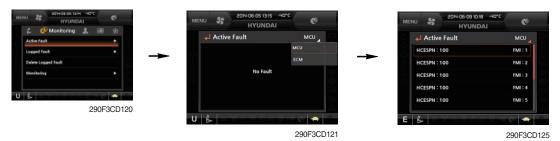
· The active faults of the MCU or engine ECM can be checked by this menu.
