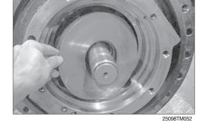
(10) Disassemble the steel ball (15) and swash piston (6) from the casing.
