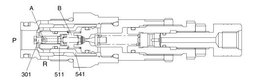
b. When the pressure in the path (P) becomes equal to the set pressure of the spring (621 or 622), the pressurized oil pushes open the poppet (611), flows around it, and flows to the low pressure path (R) through hole C.
