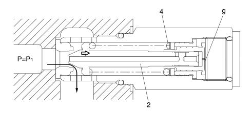
③ The oil flow chamber g via orifice m and n. When the pressure of chamber g reaches the preset force (FSP) of spring (4), the piston (7) moves left and stop the piston (7) hits the bottom of bushing (8).
