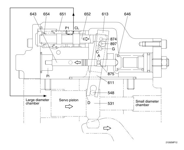
As the pilot pressure Pi decreases, the pilot piston (643) moves to the left by the action of the pilot spring (646) and causes lever 2 (613) to rotate around the fulcrum of point G. Since the pin (897) is pressed against the large hole section (C) of lever 2 by the action of the return spring (654) via the spool (652), pin (874), and feedback lever (611), the feedback lever rotates around the fulcrum of point D as lever 2 rotates, and shifts the spool to the right.
