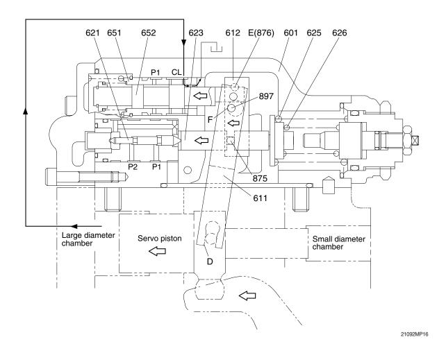
As the self pump delivery pressure P1, the compensating rod (623) is pushed back by the action of the springs (625 & 626) to rotate lever 1 (612) around point E. Rotating of lever 1 causes the feedback lever (611) to rotate around the fulcrum of point D and then the spool (652) to move to the left. As a result, port CL opens a way to the tank port.
