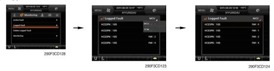
• The logged faults of the MCU or engine ECM can be checked by this menu.
