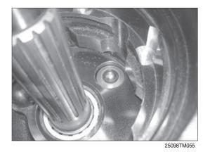
(11) Disassemble the pivot (16, 2EA) from the casing.
