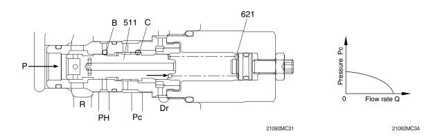
(3) The pressure at Pc1 (or Pc2) is used for the control of pump discharge flow rate, and the pump discharge flow rate can be reduced by lowering the Pc1 (or Pc2) port pressure.
