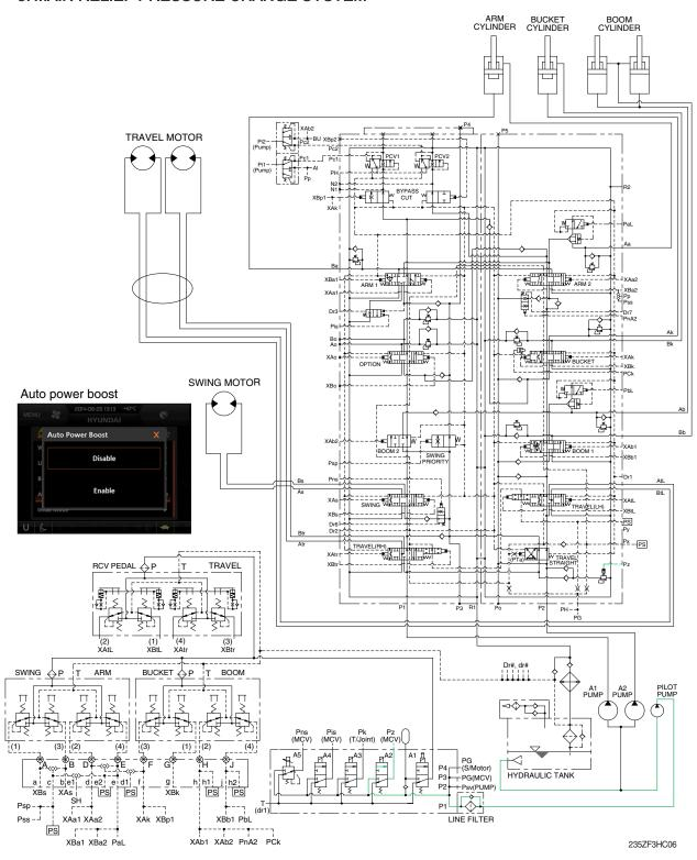
When the power boost switch on the left control lever is pushed ON, the power boost solenoid valve is actuated, the discharged oil from the pilot pump flows into **Pz** port of the main relief valve of main control valve; then the setting pressure of the main relief valve is raised from 350 kgf/cm² (4980 psi) to 380 kgf/cm² (5400 psi) for increasing the digging power.
