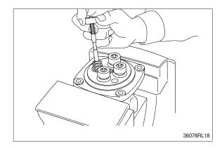
(3) Assemble O-ring (10) onto plug (8).
