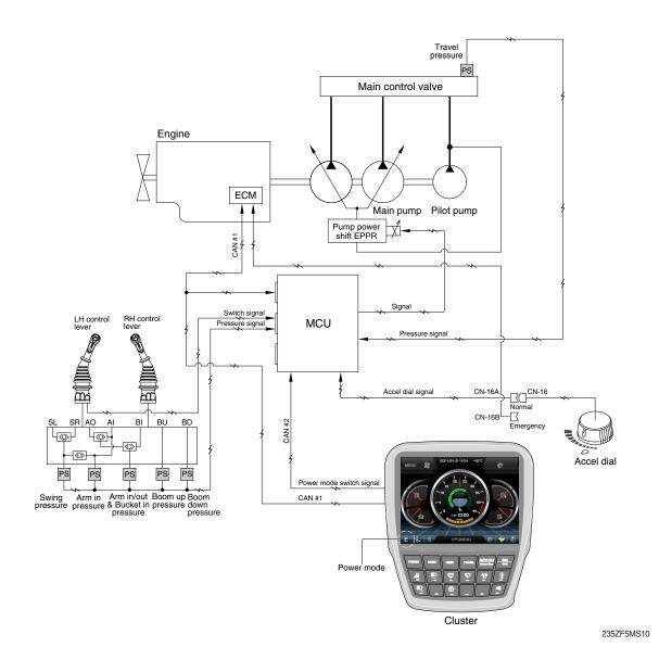
The variable power control system makes constantly exact pump control through improvement variable engine rpm control and response and optimization of control input sensor signal. It makes fuel saving.
