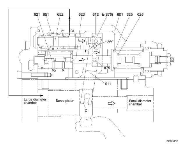
When the self pump delivery pressure P1 rises, it acts on the stepped part of the compensating piston (621). It presses the compensating rod (623) to the right till the force of the outer spring (625) and inner spring (626) balances with the hydraulic force. The movement of the compensating rod is transmitted to lever 1 (612) via pin (875).
