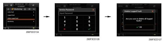
· The logged faults of the MCU or engine ECM can be deleted by this menu.
