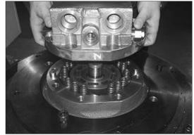
(27) Tighten the casing (1) and rear cover (34) specified torque with wrench bolt (54, 55) by using the impact wrench and torque wrench.
