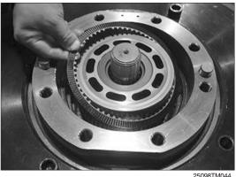
(7) Turn the casing (1) horizontal by using the assemble truck and disassemble the cylinder block kit form the casing (1).
