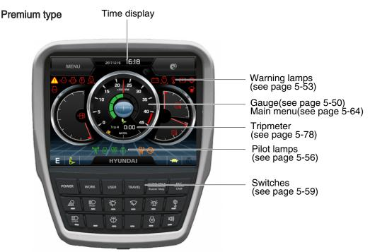
\* The warning lamp pops up and/or blinks and the buzzer sounds when the machine has a problem. The warning lamp blinks until the problem is cleared. Refer to page 3-6 for details.
