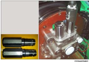
③ Using a torque wrench, disassemble plug (32) from valve casing (23) and disassemble O-ring (33, 34) and reactionless valve assy (31).
