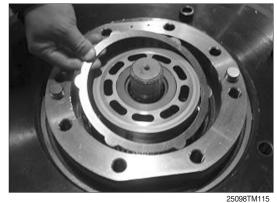
(23) Apply some grease on the D-ring and assemble it parking piston.
