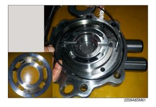
2 Using a torque wrench, disassemble relief valve (30) from valve casing (23).
