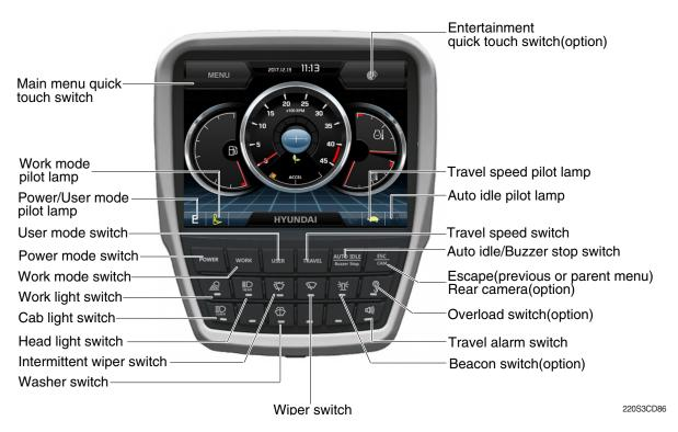
\* When some of the switches are selected, the pilot lamps are displayed on the LCD. Refer to the page 5-56 for details.
