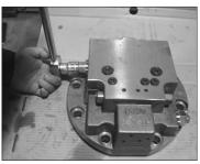
(20) Disassemble both side of the plug (48) and connector (52) from the rear cover (34) by using the torque wrench and then disassemble the spring (51), spring seat (49), parallel pin (50) and spool (47) in order.
