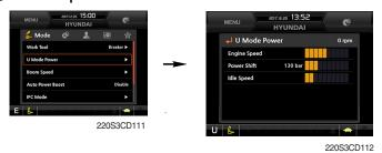
· Engine high idle rpm, auto idle rpm and pump torque (power shift) can be modulated and memorized sepa-
