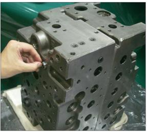
② Assemble of ball (541), spring seat (542) and spring (543): Put the O-ring (166) onto the plug (550), and tighten the plug (550) with specified torque.
