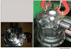
④ Disassemble spring (16) and using a jig, disassemble parking piston (15) from casing (1).
