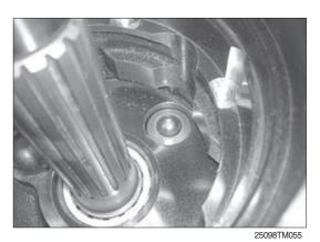
(11) Disassemble the pivot (16, 2EA) from the casing.
