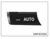
① Auto air conditiner and heater system automatically keeps the optimum condition in accordance with operator's temperature configuration sensing ambient and cabin inside temperature.
