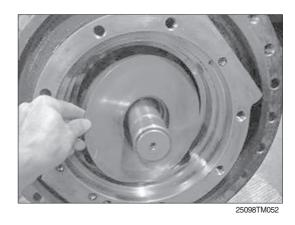
(10) Disassemble the steel ball (15) and swash piston (6) from the casing.
