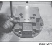
(21) Disassemble the plug (60) from the rear cover.
