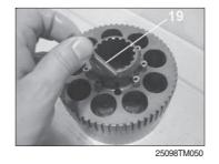
(9) Disassemble the swash plate (17) from the casing.
