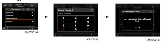
• The logged faults of the MCU, engine ECM, EPCU or air conditioner can be deleted by this menu.
