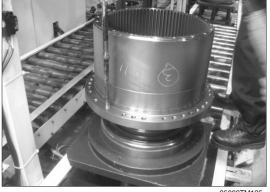
② Setting reduction unit on work stand for disassembling. Remove M16 hexagon socket head bolts that secure ring gear and housing assembly.
