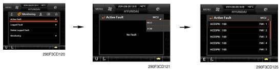
· The active faults of the MCU, engine ECM or air conditioner can be checked by this menu.
