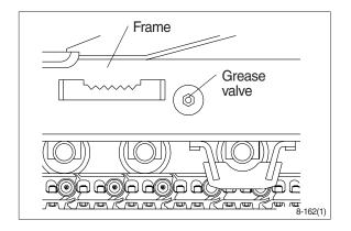
(2) Jack up the track link height enough to permit carrier roller removal.
