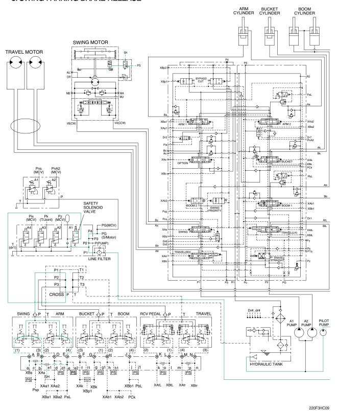
When the swing control lever or arm in lever is tilted, the pilot oil flows into SH port through shuttle valve
