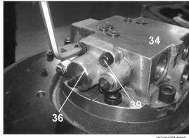
(2) Disassemble the wrench bolt (54, 55) to tighten the casing (1) and rear cover (34) by using the L-wrench or impact wrench.
