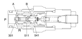
b. When the pressure in the path (P) exceeds the set pressure of the spring (621 or 622), the pressurized oil pushes open the poppet (611), flows around it, and flows to the low pressure path (R) through hole C.
