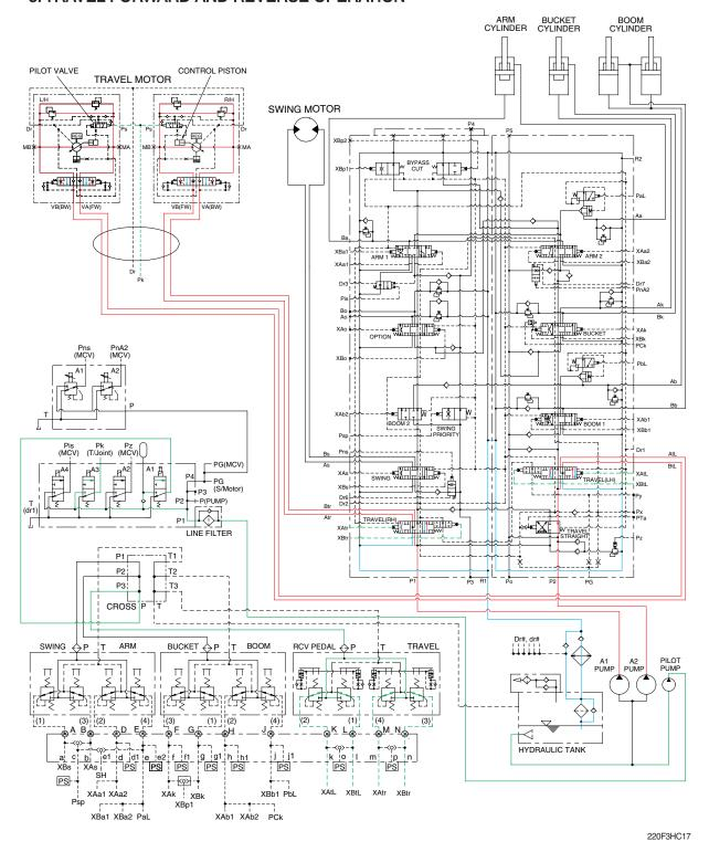
When the travel levers are pushed forward or reverse position, the travel spools in the main control valve are moved to the forward or reverse travel position by the pilot oil pressure (XAtr, XBtr, XAtL, XBtL) from the remote control valve.
