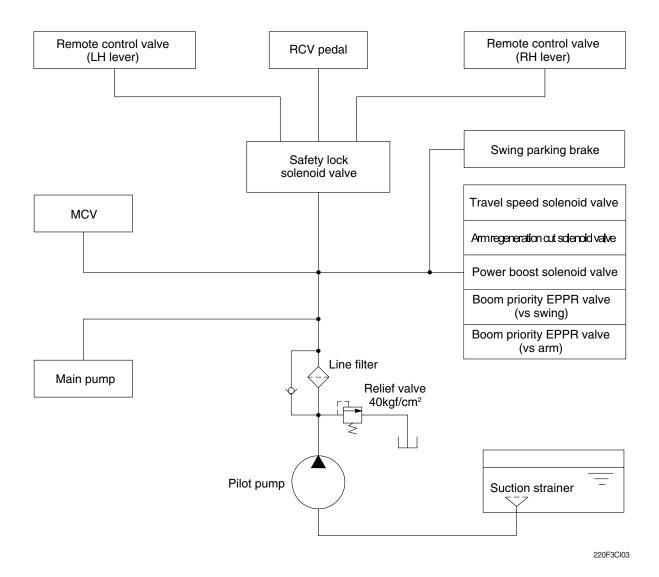
The pilot circuit consists of suction circuit, delivery circuit and return circuit.
