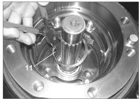
(13) Disassemble the shaft (8) from the casing (1).
