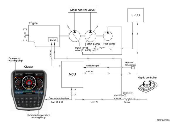
1. If the engine coolant temperature or the hydraulic oil temperature is overheated over 100°C, the warning lamp is ON and the pump input torque or the engine speed is reduced as below logic table.
