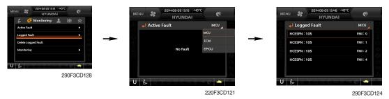
• The logged faults of the MCU, engine ECM, EPCU or air conditioner can be checked by this menu.
