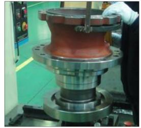
(3) Put taper bearing into it. Rotate bearing by hands for checking after assembly.
