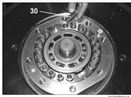
(5) Disassemble the parking piston (25) by using the jig for disassembling parking piston.
