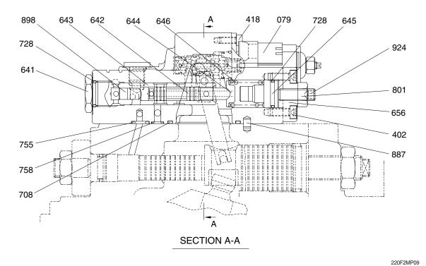
402 Hexagon socket screw 645 Adjust stem (Q) 758 Square ring 418 Hexagon socket screw 646 Pilot spring 801 Nut 641 Pilot plug 656 Cover 887 Pin 642 Pilot spool 708 O-ring 898 Piston piston 432 Pilot sleeve 728 O-ring 924 Set screw 644 Spring seat (Q) 755 O-ring
