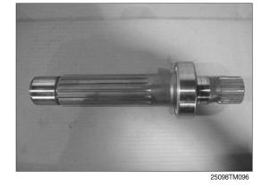
(14) Assemble the heat-fitted shaft (8) into casing (1).
