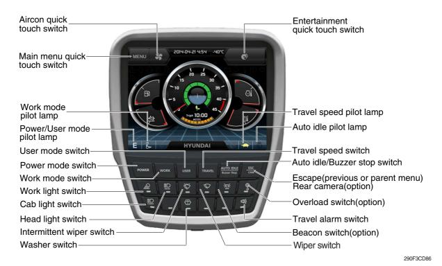
When some of the switches are selected, the pilot lamps are displayed on the LCD. Refer to the page 5-94 for details.
