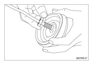
(14) Pull out cord and tube through adjusting nut hole provided in direction 60 °to 120 °from casing hole.
