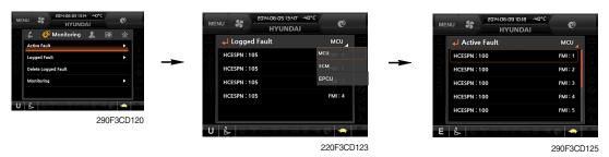
• The active faults of the MCU, engine ECM, EPCU or air conditioner can be checked by this menu.
