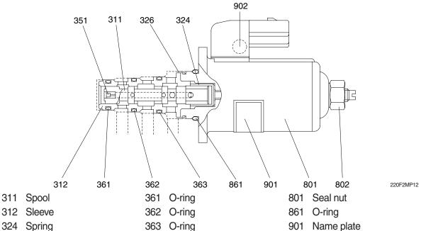
324 Spring326 Retaining ring351 Orifice
