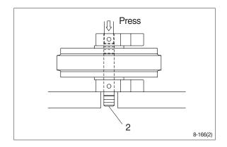
⑥ Remove the bushing (4) from idler, using a special tool.
