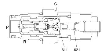
c. Opening of the poppet (611) causes the pressure in Chamber B to fall and the plunger (511) to open. As the result the pressurized oil in the path (P) runs into the low pressure path (R) directly.
