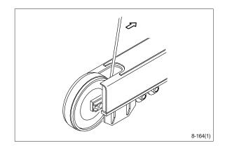
(2) Sling the recoil spring (1) and pull out idler and recoil spring assembly from track frame, using a pry.
