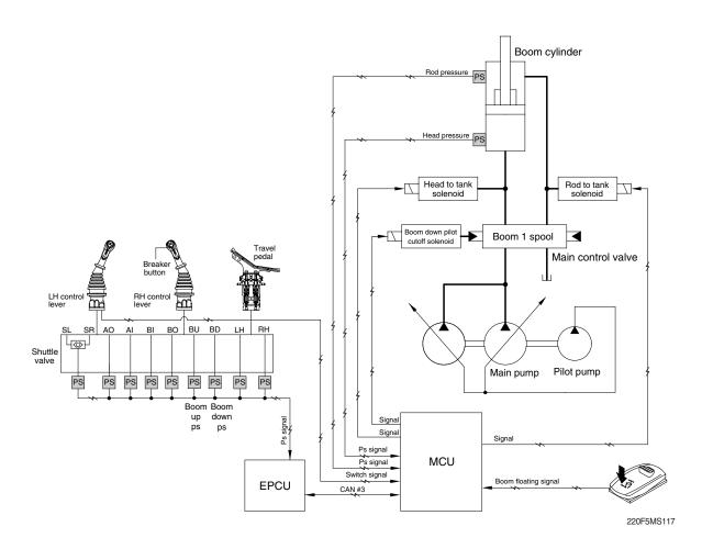
Boom floating automatically controls boom cylinder along the ground by operating arm cylinder only.
