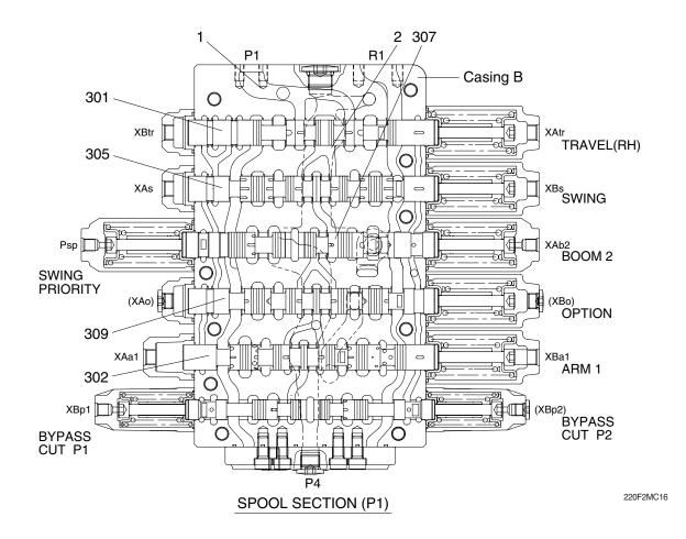
When all spools are in the neutral positions, the pressurized oil discharged from the hydraulic pump (A1) passes through Port P1, the main path (1), the bypass circuit (2) passing the spools for travel right (301), swing (305), boom confluence (boom 2; 307), option (309) and arm 1 (302), and returns to the hydraulic oil tank through the tank port (R1).
