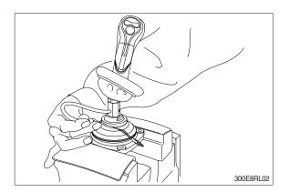
(4) Loosen lock nut (22) and adjusting nut (17) with spanners on them respectively, and take out handle section as one body.
