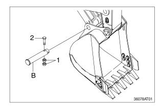
3 Remove nut (3), bolt (4) and draw out the pin (B).
