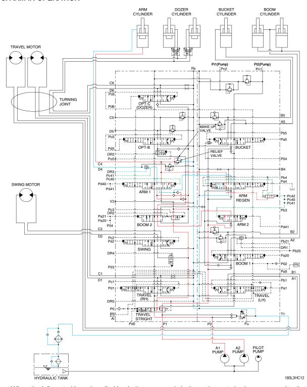
When the left control lever is pulled back, the arm spools in the main control valve are moved to the roll in position by the pilot oil pressure from the remote control valve.
