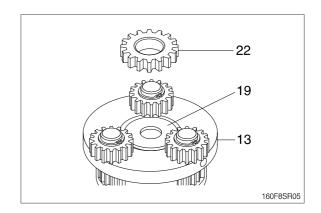
(9) Assemble carrier 1 (13) assembly onto the carrier 2 (7) assembly.
