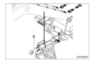
⑤ Disconnect boom cylinder hoses (7) and put plugs on cylinder pipe.
