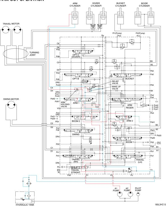
When the left control lever is pushed forward, the arm spools in the main control valve are moved to the roll out position by the pilot oil pressure from the remote control valve.
