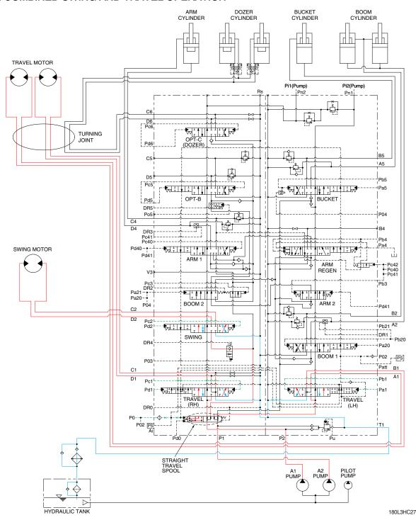
When the swing and travel functions are operated simultaneously, the swing spool and travel spools in the main control valve are moved to the functional position by the pilot oil pressure from the remote control valve and straight travel spool is pushed to the right by the pilot oil pressure from the pilot pump.
