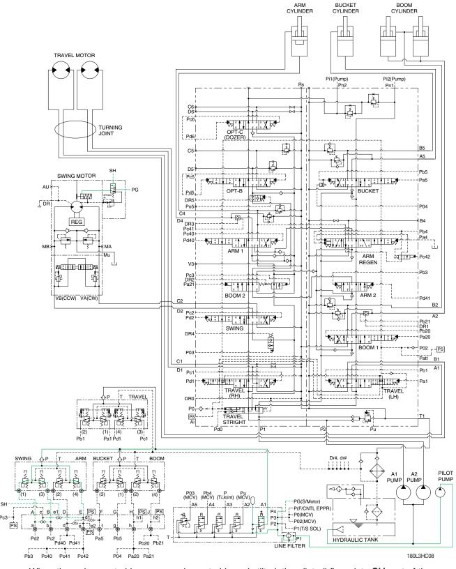
When the swing control lever or arm in control lever is tilted, the pilot oil flows into **SH** port of time delay valve.
