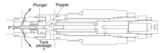
(4) The pressure at port P becomes lower than set pressure of the spring, the poppet is seated by spring force. Then the pressure at port P becomes equal to set pressure of the spring and the plunger is seated to the socket.
