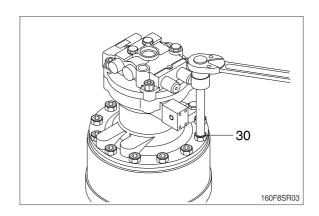
(3) Tighten 3 M16 eye bolts to the ring gear (6) and then lift the ring gear (6) out of the casing (1).
