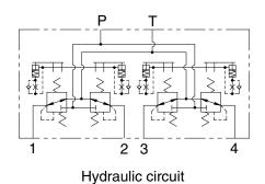
Port Port size Port Ρ Pilot oil inlet port Τ Pilot oil return port Travel (LH, Forward) 1 PF 1/4 2 Travel (LH, Backward) 3 Travel (RH, Forward) 4 Travel (RH, Backward)
