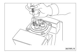
(4) Assemble O-ring (14) onto plug (13).
