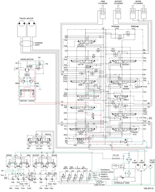
When the left control lever is pushed left or right, the swing spool in the main control valve is moved to the left or right swing position by the pilot oil pressure from the remote control valve.
