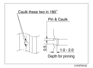
(3) Install No.2 pin (90-5) into No.2 carrier where the holes for No.2 pin (90-5) are to be in line with those of No.2 carrier, and then, install spring pins into the holes.
