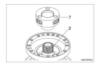
(6) Assemble sun gear 2 (12) to the center of the carrier 2 (7) assembly.
