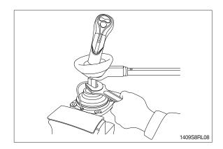
(18) Apply grease to rotating section of joint and contacting faces of disk and push rod.
