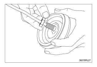
(15) Pull out cord and tube through adjusting nut hole provided in direction 60° to 120° from casing hole.
