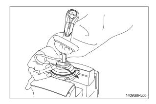
(4) Loosen lock nut (21) and adjusting nut (20) with spanners on them respectively, and take out handle section as one body.
