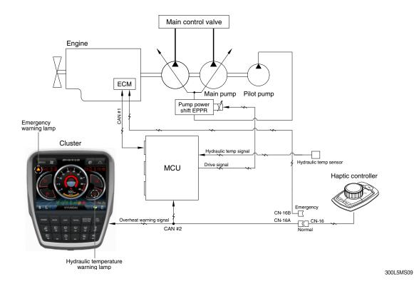
1. If the engine coolant temperature or the hydraulic oil temperature is overheated over 100°C, the warning lamp is ON and the pump input torque or the engine speed is reduced as below logic table.
