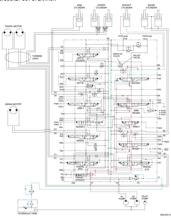
When the right control lever is pushed right, the bucket spool in the main control valve is moved to the roll out position by the pilot oil pressure from the remote control valve.
