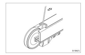
(2) Sling the recoil spring (1) and pull out idler and recoil spring assembly from track frame, using a pry.
