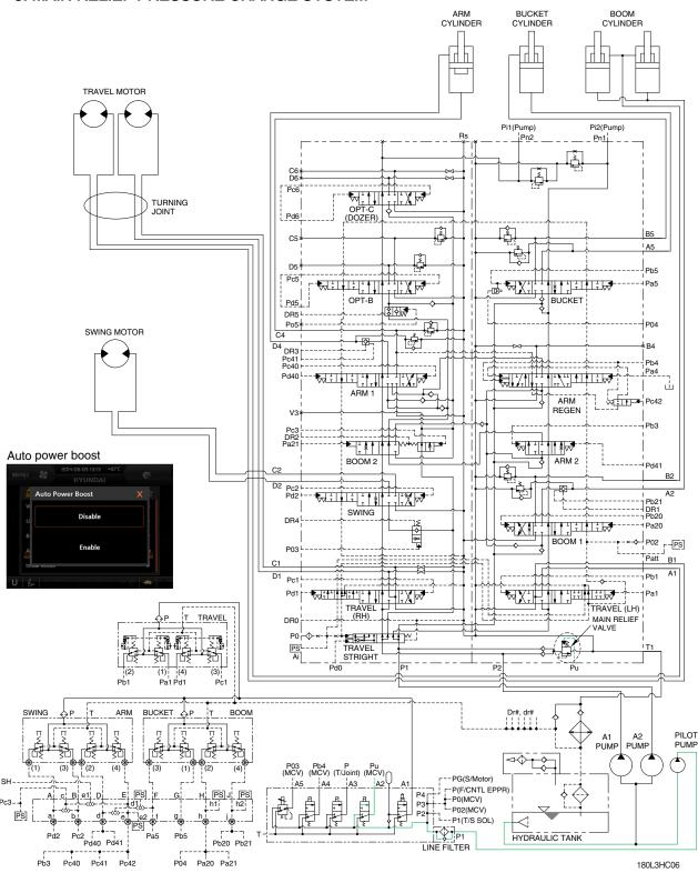
When the power boost switch on the left control lever is pushed ON, the power boost solenoid valve is actuated, the discharged oil from the pilot pump flows into **Pu** port of the main relief valve of main control valve; then the setting pressure of the main relief valve is raised from 350 kgf/cm² (4980 psi) to 380 kgf/cm² (5400 psi) for increasing the digging power.
