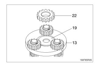
(5) Tighten two M10 eye bolts to carrier 1 (13) and lift up and remove carrier 1 (13) as subassembly.
