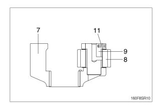
(5) Assemble carrier 2 (7) assembly correctly to the drive shaft (2).
