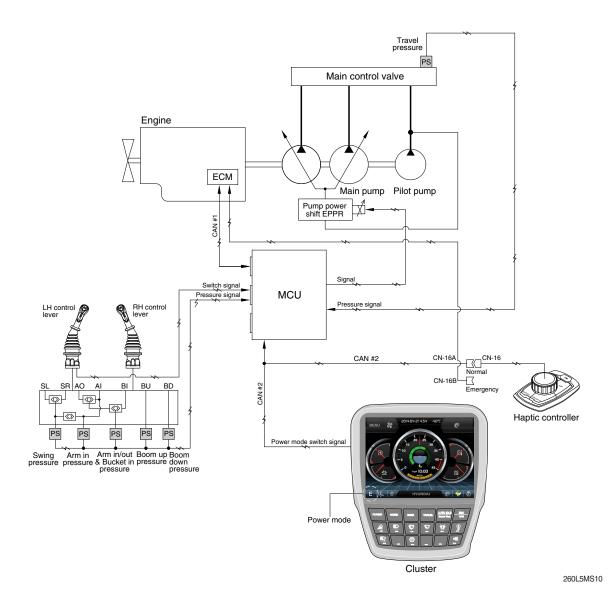
The variable power control system controls the engine and pump mutual power according to RCV lever stroke and pump load.
