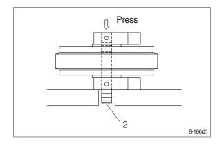
⑥ Remove the bushing (4) from idler, using a special tool. Only remove bushing if replacement is necessity.
