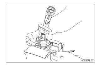
(17) Determine handle direction, tighten lock nut (22) to specified torque to fix handle.
