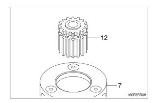
(8) Remove carrier 2 (7) assembly from casing (1).
