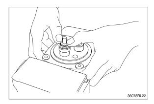
(8) When return spring is strong in force, assemble 4 sets at the same time, utilizing plate (16), and tighten joint (18) temporarily.
