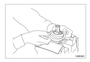
(14) Fit boot (25) and lock nut (21), and handle subassembly is assembled completely.
