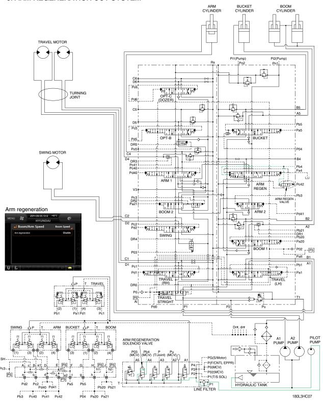
When the arm regeneration is selected to disable on the cluster, the arm regeneration solenoid valve is activated. The pilot oil from pilot pump flow into **Pb4** port in main control valve through solenoid valve and the arm regeneration spool is shifted to left.
