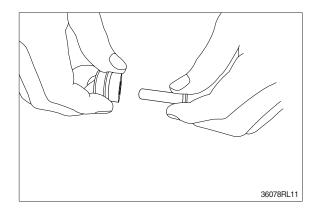
(14) Remove O-ring (14) and seal (15) from plug (13).
