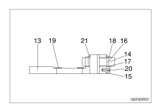
(8) Install sun gear 1 (22) onto the side plate 3 (19).
