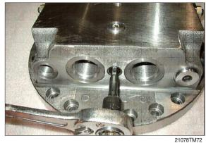
19) Assemble plug (62, 63) into rear cover (29) and assemble relief valve assembly.
