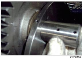
(3) Install No.1 pin (91-5) into No.1 carrier where the holes for No.1 pin (91-5) are to be in line with those of No.1 carrier, and then, install spring pins into the holes.
