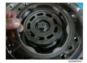
(7) Remove the cylinder block kit (II).※ It is easier to work by placing the shaft casing (1) horizontal.
