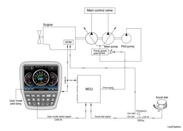
1) Engine speed, idle speed and pump power shift pressure can be adjusted and memorized in the U-mode.
