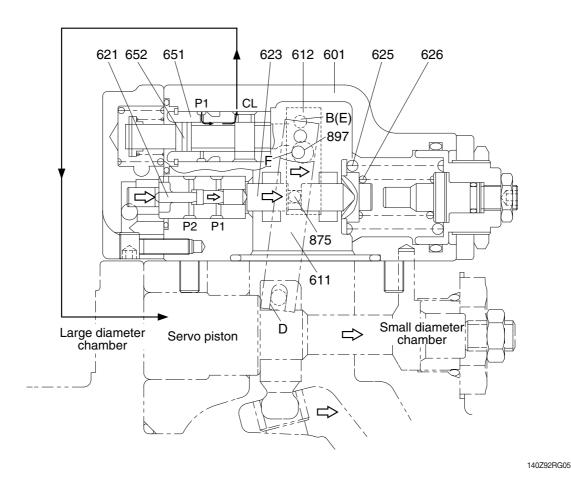
The set horsepower valve is shifted by varying the command current level of the proportional pressure reducing valve attached to the pump.
