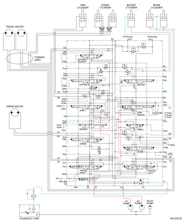
When the boom up and bucket functions are operated simultaneously, each spool in the main control valve is moved to the functional position by the pilot oil pressure from the remote control valve.
