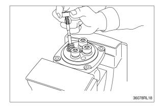
(3) Assemble O-ring (10) onto plug (8).
