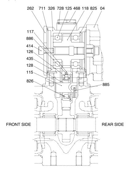
04 Gear pump 128 Bearing spacer 711 O-ring 115 Shaft 262 Cover 728 O-ring 117 Gear No. 2 326 Gear case 825 Retainer ring 118 Gear No. 3 414 Hexagon socket bolt 826 Retainer ring 125 Ball bearing 435 Flange socket bolt 885 Spring pin 468 Plug 886 Pin 126 Roller bearing
