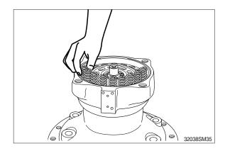
(13) When assembling the needle bearing (21), insert the needle bearing (21) into rear cover (20) by hammering.
