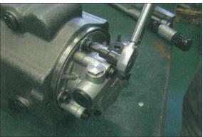
(11) Attach the PTO unit (05) by fastening the flange socket (435) to the valve block (312).
