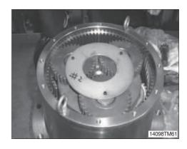
(4) Remove planetary gear R (117), needle bearing, inner race (119) and holder (116) from hub (105).
