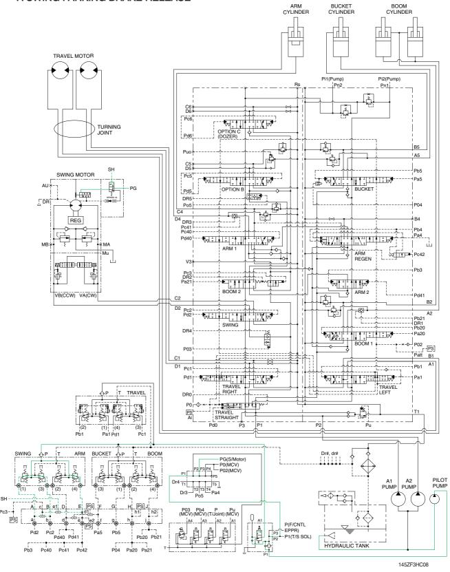
When the swing control lever or arm in control lever is tilted, the pilot oil flows into SH port through shuttle valve.
