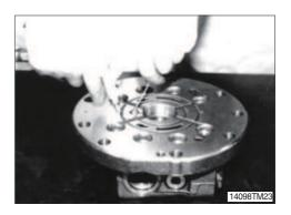
Remove the valve (19) and spring (20) from rear flange (1) downside hole with shaking lightly.
