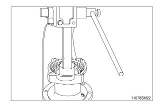
(2) Install the roller bearing (3) to the drive shaft (5).
