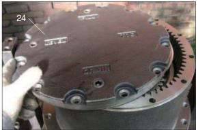
(13) Tighten wrench bolt (25) using a air impact.
