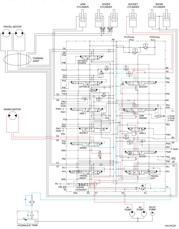
When the swing and bucket functions are operated simultaneously, the swing spool and bucket spool in the main control valve are moved to the functional position by the pilot oil pressure from the remote control valve.
