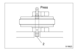
© Remove the bushing (4) from idler, using a special tool.
