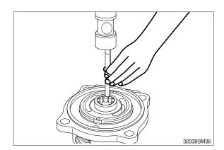
(14) Reassemble valve plate (23) to the rear cover (20) and reassemble O-ring (18).
