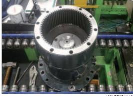
(30) Assemble carrier No.2 sub assembly.
