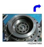
(10) Put O-ring (23) into shaft casing (1). Apply the grease to O-ring.
