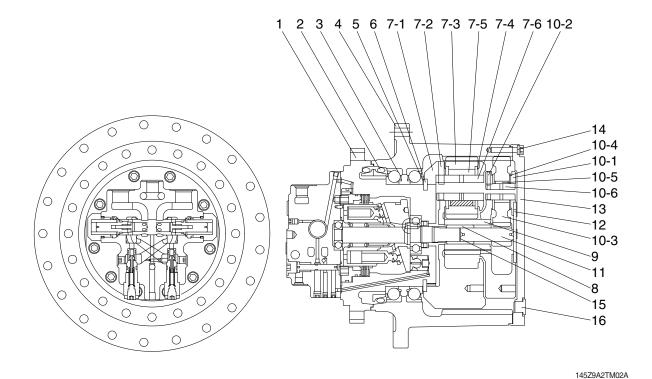
Spindle 7-4 Washer 2 10-5 Bearing 1 1 10-6 Pin 1 2 Floating sesal 7-5 Bearing 2 3 Ball bearing 7-6 Pin 2 11 Sun gear 1 4 Housing 8 Coupling Plate 1 12 5 Shim 9 Sun gear 2 Cover 13 6 Shim 10 Carrier assy 1 14 Bolt 7 Carrier assy 2 10-1 Carrier 1 Snap ring 7-1 Carrier 2 10-2 Spring pin 1 Plug 16 7-2 Spring pin 2 10-3 Planetary gear 1
