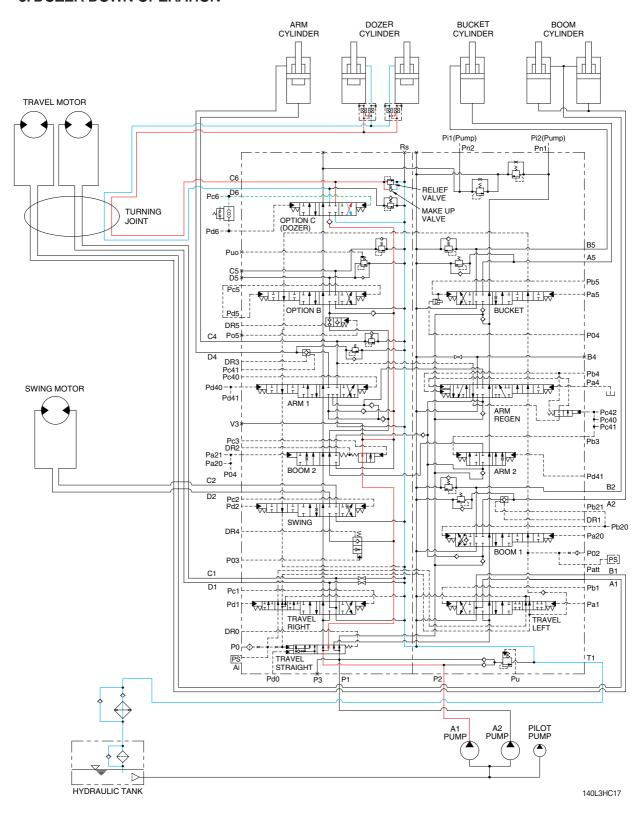
When the dozer control lever is pushed forward, the dozer spool in the main control valve is moved to the dozer down position by the pilot oil pressure from the remote control valve.
