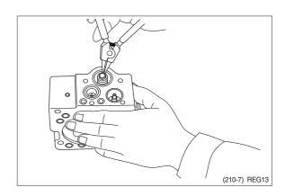
compensating piston (621) and piston case (622) into compensating hole. Fit pilot cover (641) and tighten it with hexagonal socket head screws (437, 438).
