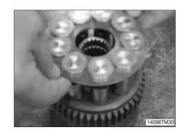
② Piston (5) and shoe (6) from the removed retainer plate (7).
