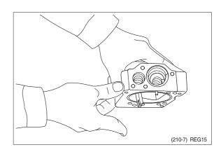
(13) Install cover (C, 629) fitted with adjusting screws (628), adjusting ring (C, 627), lock nut (630), hexagon nut (801) and adjusting screw (924).
