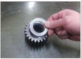
(17) Disassemble needle bearing No.2 (12). (3 pcs)
