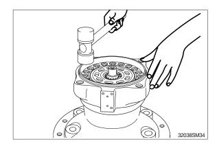
(12) Reassemble brake spring (19) to the brake piston (16).
