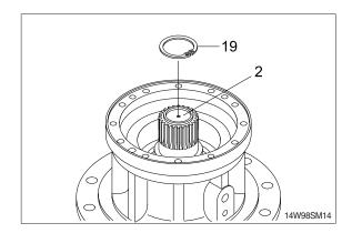
(11) Remove drive shaft (2) with roller bearing(6) and oil seal (7) assembled.Remove knock pin (22) from the casing(1).
