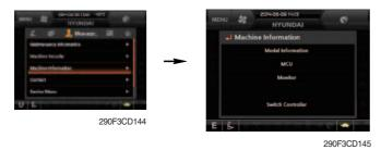
· This can confirm the identification of the model information (ECU), MCU, monitor, switch controller, RMCU, relay driver unit, FATC (air conditioner controller), AAVM (opt).
