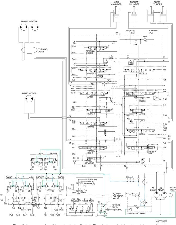
The pilot pump receive oil from the hydraulic tank. The discharged oil from the pilot pump flows to the safety solenoid valve. The oil is filtered by the line filter.
