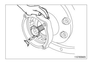
(5) Insert the shoe plate (8) with the body (1) position horizontally.
