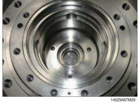
(14) Disassemble valve plate (51) and ball bearing (49) from valve casing (25).
