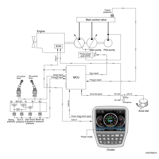
The new variable power control system makes constantly exact pump control through improvement variable engine speed control and response and optimization of control input sensor signal.
