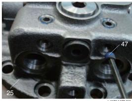
(16) Disassemble plug (37) from valve casing (25) using a torque wrench and disassemble two speed control spool (35), spring (36) in regular sequence.
