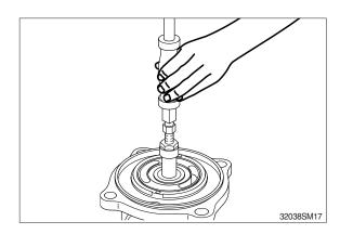
(16) When disassembling the relief valve, release the adjusting screw (5).
