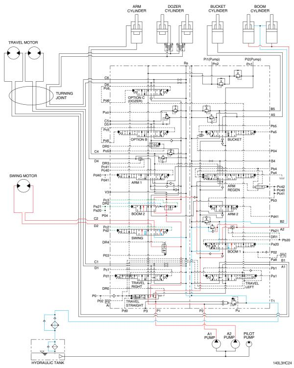
When the swing and boom up functions are operated simultaneously, the swing spool and boom spools in the main control valve are moved to the functional position by the pilot oil pressure from the remote control valve.
