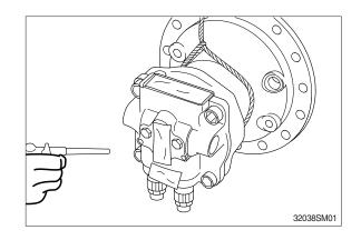
(2) Loosen the drain plug to discharge oil in the body(1).
