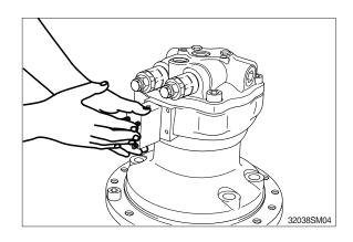
(5) Remove the relief valve (30) from rear cover (20).
