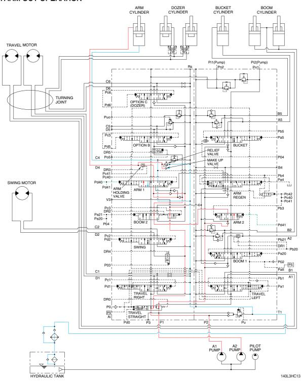
When the left control lever is pushed forward, the arm spools in the main control valve are moved to the arm out position by the pilot oil pressure from the remote control valve.
