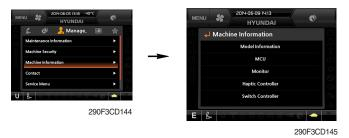
· This can confirm the identification of the model information (ECU), MCU, monitor, haptic controller, switch controller, RMCU, relay driver unit, FATC (air conditioner controller), AAVM (opt).
