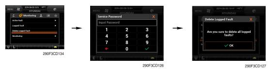
· The logged faults of the MCU, engine ECM or air conditioner can be deleted by this menu.
