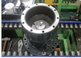
(30) Assemble carrier No.2 sub assembly.
