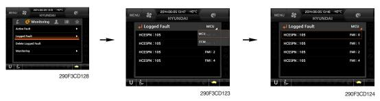
• The logged faults of the MCU, engine ECM or air conditioner can be checked by this menu.
