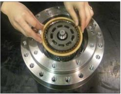
(11) Insert back-up ring & O-ring in parking piston.
