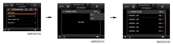
· The active faults of the MCU, engine ECM or air conditioner can be checked by this menu.
