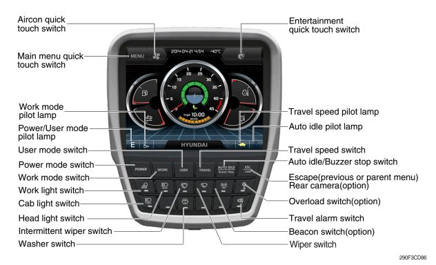
When some of the switches are selected, the pilot lamps are displayed on the LCD. Refer to the page 5-77 for details.
