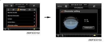
· When the machine is on the flatland, if tap the "initialization", the values of X, Y reset "0".
