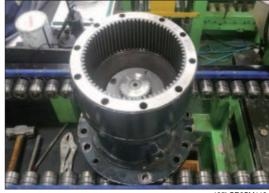
(30) Assemble carrier No.2 sub assembly.
