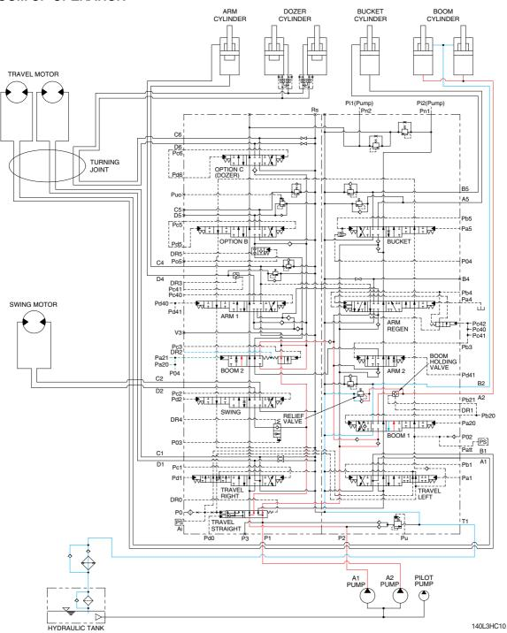
When the right control lever is pulled back, the boom spools in the main control valve are moved to the up position by the pilot oil pressure from the remote control valve.
