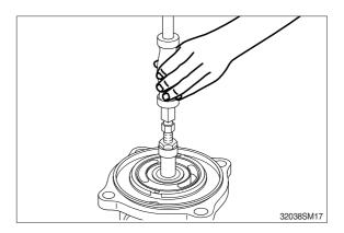
(16) When disassembling the relief valve, release the adjusting screw (5).
