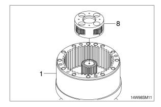
(8) Assemble sun gear 2 (14) and side plate 1 (26) to the center of the carrier 2 assembly (8).
