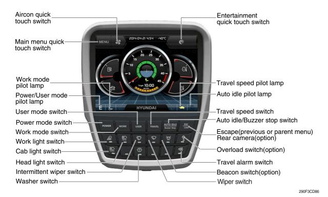
When some of the switches are selected, the pilot lamps are displayed on the LCD. Refer to the page 5-71 for details.
