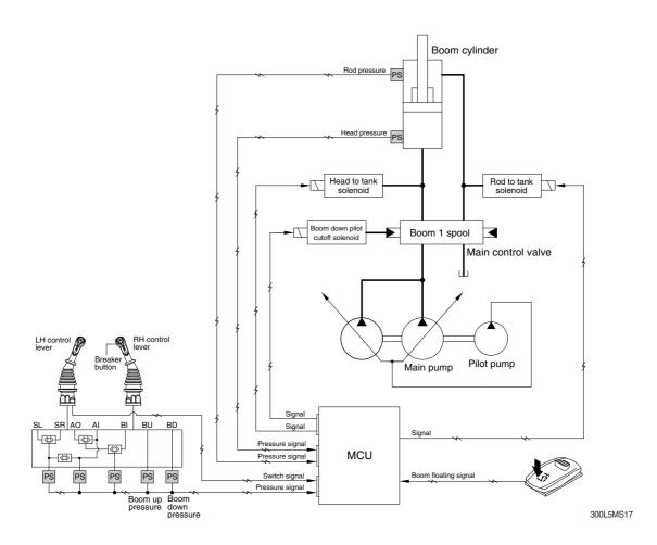
Boom floating automatically controls boom cylinder along the ground by operating arm cylinder only.
