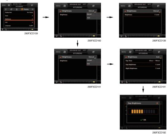
· If "Auto" is chosen, brightness for day and night can be differently set up. Also by using the bar in lower side, users can define which time interval belongs to day and night. (in bar figure, white area represents night time while orange shows day time)
