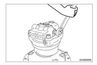
(7) Remove rear cover (20) from body (1). Then, remove the valve plate (23) from rear cover (20) with care.
