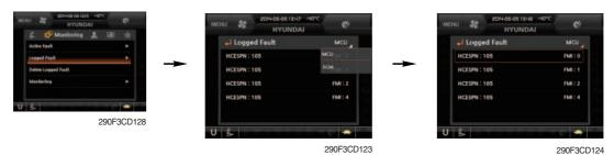
• The logged faults of the MCU, engine ECM or air conditioner can be checked by this menu.
