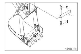
Remove nut (3), bolt (4) and draw out the pin ( ) then remove the bucket assembly.Weight: 480 kg (1060 lb)
