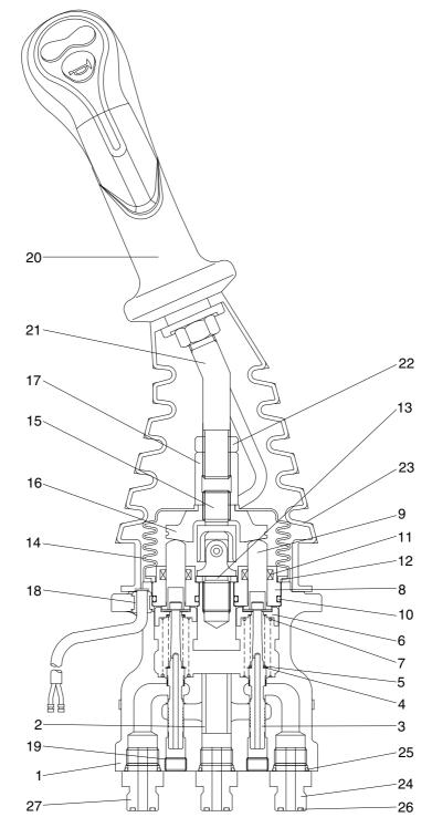
Plug Case Joint assembly 22 Nut 1 8 15 Swash plate 2 Bushing 9 Push rod 16 23 Boot Adjusting nut Last guard filter 3 Spool 10 O-ring 17 24 Bushing 4 Shim 11 Rod seal 18 25 O-ring Plate 5 Spring 12 19 Plug 26 O-ring 6 Spring seat Spacer Handle assembly 27 Connector 13 20 7 Boot 21 Handle bar Spring 14
