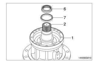
(3) Install stop ring (25) on top of drive shaft (2).
