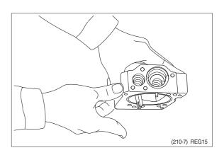
(13) Install cover (C, 629) fitted with adjusting screws (628), adjusting ring (C, 627), lock nut (630), hexagon nut (801) and adjusting screw (924).
