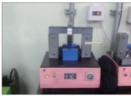
(19) Shrink fit taper bearing (3) on drive shaft, complete drive shaft sub assembly.
