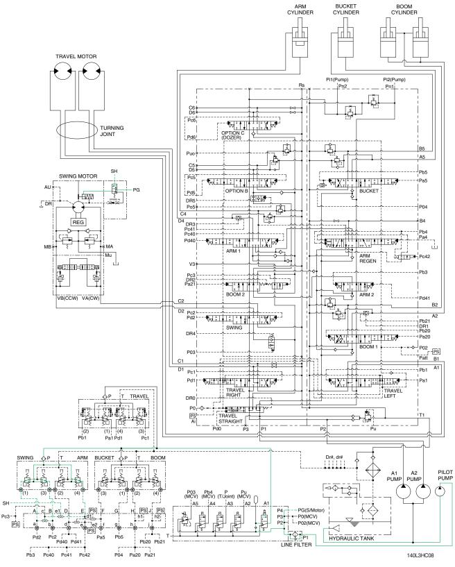
When the swing control lever or arm in control lever is tilted, the pilot oil flows into SH port through shuttle valve.
