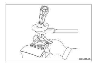
(17) Apply grease to rotating section of joint and contacting faces of disk and push rod.
