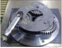
6) First, place bearing (2) on the ring gear (1), then put jig on it, then press it with press machine.
