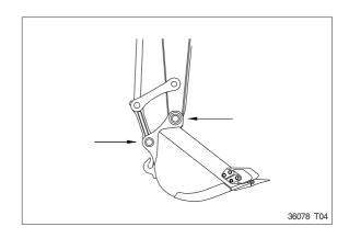
② Remove nut (1), bolt (2) and draw out the pin ( ).
