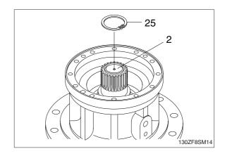
(11) Remove drive shaft (2) with roller bearing(6) and oil seal (7) assembled.Remove knock pin (28) from the casing (1).
