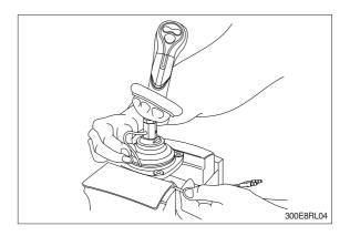
(16) Determine handle direction, tighten lock nut (22) to specified torque to fix handle.
