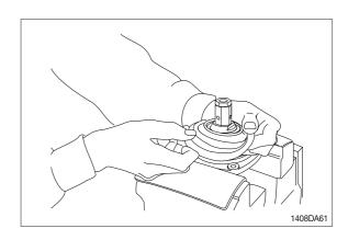
(13) Fit boot (23) and lock nut (22), and handle subassembly is assembled completely.
