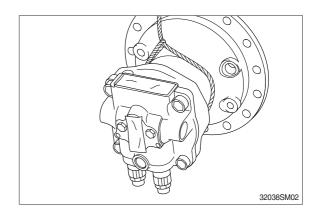
(3) Fix the drive shaft (5) on the workbench with the end of output shaft down. Put matching marks on body (1) and valve rear cover (20) for easy reassembly.
