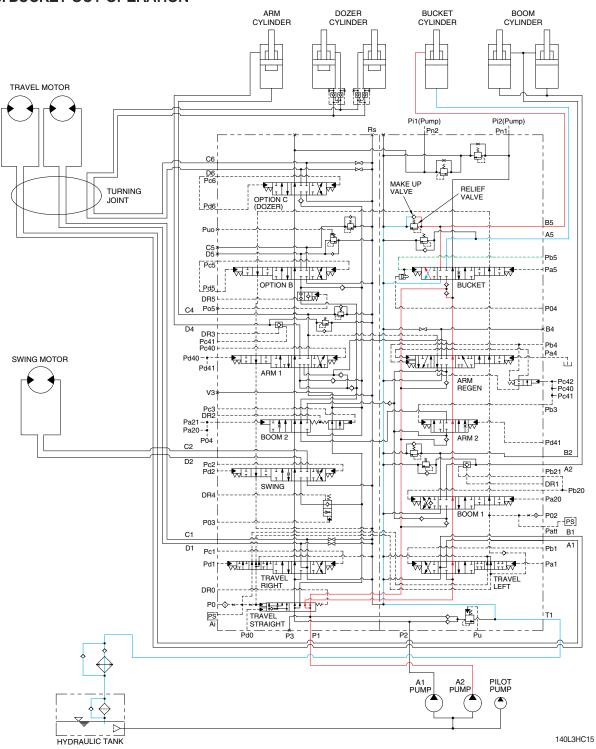
When the right control lever is pushed right, the bucket spool in the main control valve is moved to the bucket out position by the pilot oil pressure from the remote control valve.
