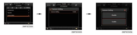
· In the operation screen, rear camera screen show up when ESC/CAM button is pushed.
