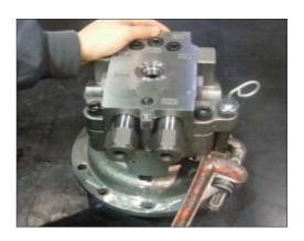
(4) Disassemble two sets of relief valve assembly (31) using 36 mm socket wrench.
