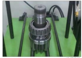
(22) Disassemble taper bearing (3) and oil seal (27) by using a press machine.
