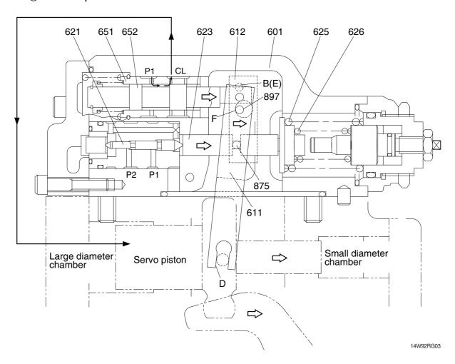
When the self pump delivery pressure P1 or the companion pump delivery pressure P2 rises, it acts on the stepped part of the compensating piston (621). It presses the compensating rod (623) to the right till the force of the outer spring (625) and inner spring (626) balances with the hydraulic force. The movement of the compensating rod is transmitted to lever 1 (612) via pin (875).
