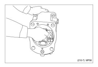
(12) Tapping lightly shaft ends of drive shafts (111, 113) with plastic hammer, take out drive shafts from swash plate supports.
