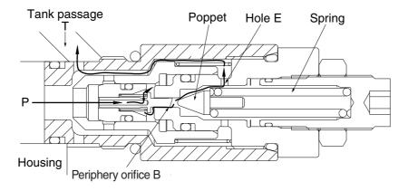
(3) Opening of the poppet causes the pressure in chamber A to fall and the plunger to open. As the result the pressurized oil at port P runs into tank passage (T).
