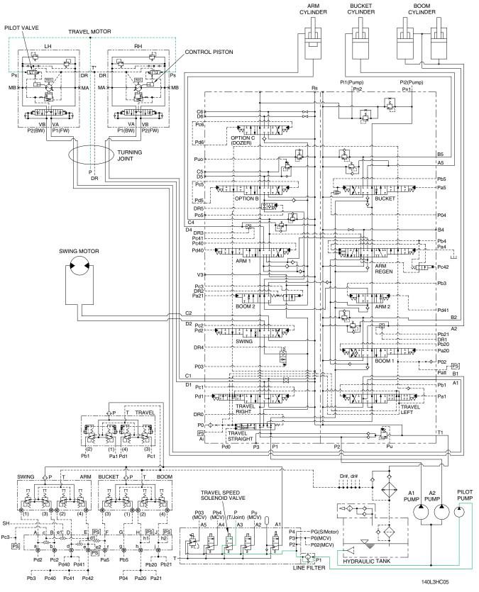
When the travel speed solenoid valve was placed in the Hi position, the pressure oil from pilot pump through line filter flows to port **Ps** of travel speed change over valve, and the control piston is pushed up, thus minimizing the displacement.
