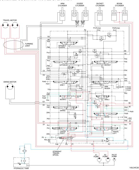
When the boom and travel functions are operated simultaneously, the boom spools and travel spools in the main control valve are moved to the functional position by the pilot oil pressure from the remote control valve and the straight travel spool is pushed to the right by the oil pressure from pilot pump.
