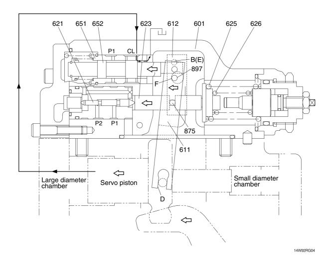
As the self pump delivery pressure P1 or the companion pump delivery pressure P2 decreases, the compensating rod (623) is pushed back by the action of the springs (625 & 626) to rotate lever 1 (612) around point E. Rotating of lever 1 causes the feedback lever (611) to rotate around the fulcrum of point D and then the spool (652) to move to the left. As a result, port CL opens a way to the tank port.
