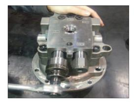
(5) Unscrew socket bolt (42) (4EA) using 12 mm hexagon wrench.
