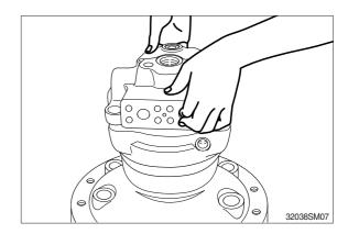
(8) Remove the brake spring (19) from brake piston (16).
