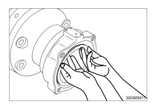
(12) Remove snap ring (4) and remove drive shaft (5) from body (1).
