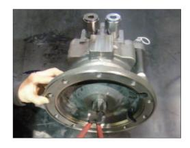
(3) Disassemble level gauge assembly (41) using pipe wrench.
