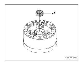
(4) Tighten two M10 eye bolts to carrier 1 assy (15) and lift up and remove carrier 1 (15) as subassembly.
