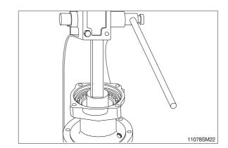
(2) Install the roller bearing (3) to the drive shaft (5).
