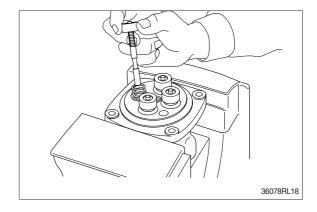
(3) Assemble O-ring (10) onto plug (8).
