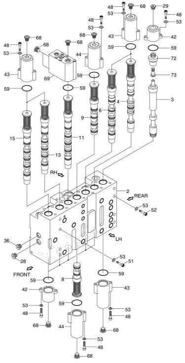
Option C spool assy 2 Housing-P2 51 Socket head bolt 15 3 Straight travel spool assy 28 Plug 52 Socket head bolt 4 Travel spool assy 29 Plug 53 Spring washer 6 Swing spool assy 36 Plug 59 O-ring 8 Swing priority spool assy 42 Pilot cover A Dust cap 68 9 TS sleeve Boom 2 spool assy 43 Pilot cover B1 72 11 Arm 1 spool assy 44 Pilot cover B2 73 TS piston 13 Option B1 spool assy 48 Socket head bolt
