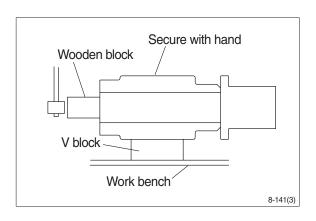
(5) Remove seventeen slipper seal (6), O-ring (7, 8) and wear ring (11) from hub (1).
