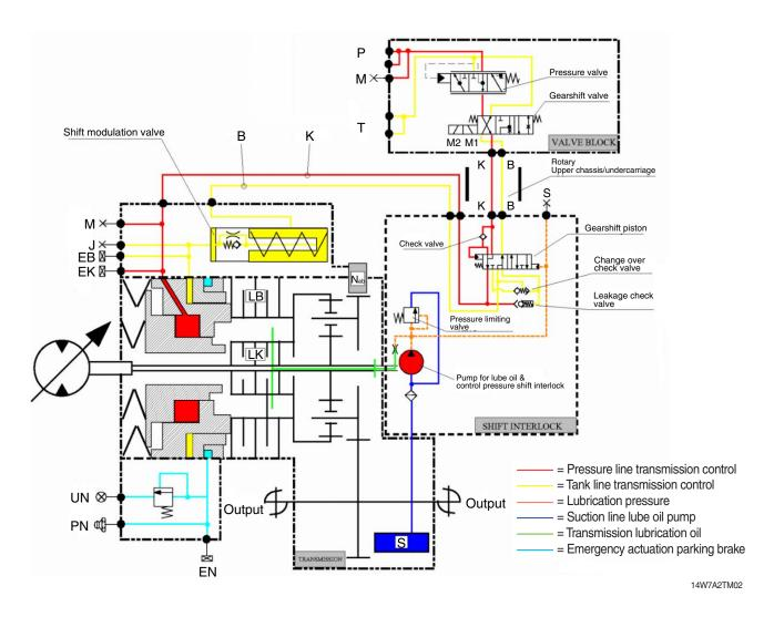
Measuring points-Transmission/Shift interlock:
