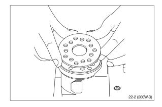
(24) Guide the cardan shaft down into the bore so that the slot is parallel with the connection flange.
