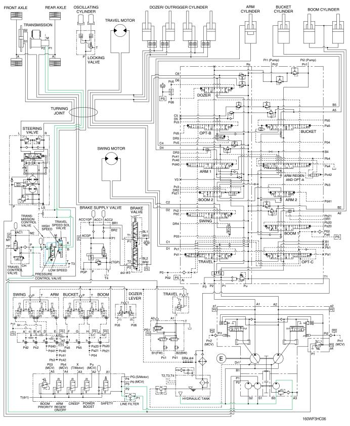
When RH multifunction switch was turned to high or low speed position, the pressure oil from pilot pump flows to travel speed solenoid valve through pressure control valve, thus the transmission is changed into high (P1) or low (P2) speed condition.
