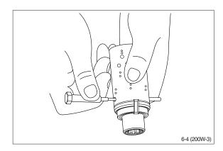
\* A small mark has been made with a pumice stone on both spool and sleeve close to one of the slots for the neutral position spring as figure.
