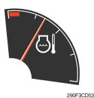
① This gauge indicates the temperature of coolant.
