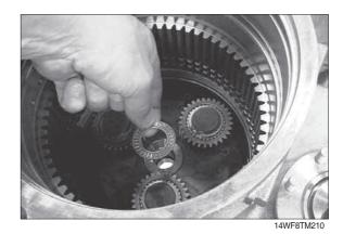
23) Insert preassembled input shaft (with ring
