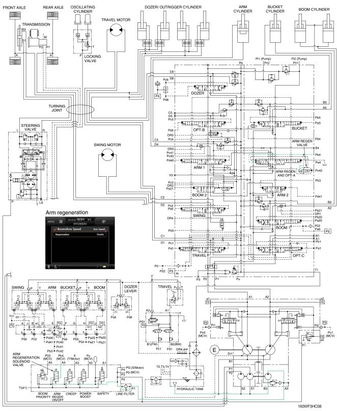
When the arm regeneration function is selected to **Disable** on the cluster, the arm regeneration solenoid valve is activated. The pilot oil from pilot pump flows into **Pb4** port in main control valve through solenoid valve and the arm regeneration spool and arm regeneration valve are shifted to right. Then, the oil from arm regeneration passage returns to tank and the arm regeneration function is deactivated.
