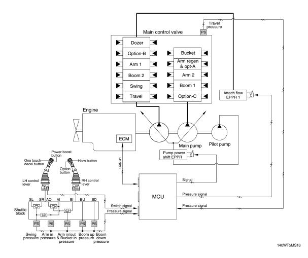
1. When the requirement of pump flow rate is low, IPC mode controls pump flow rate to improve fuel efficiency.
