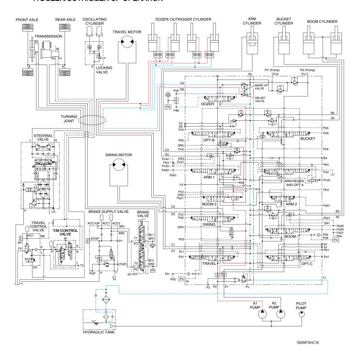
When the dozer control lever is pulled back, the dozer spool in the main control valve is moved to the dozer up position by the pilot oil pressure from the remote control valve.
