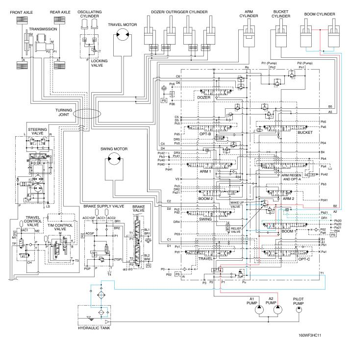
When the right control lever is pushed forward, the boom 1 spool in the main control valve is moved to the down position by the pilot oil pressure from the remote control valve.
