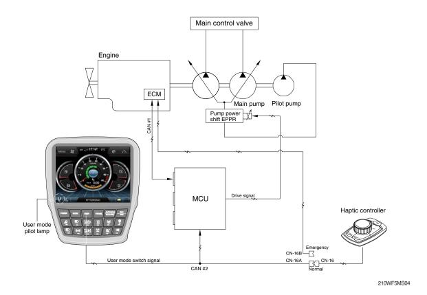
1) High idle rpm, auto idle rpm and EPPR pressure can be adjusted and memorized in the U-mode.
