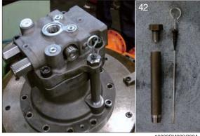
① Assemble time delay valve assy (33) into rear cover (21) with a wrench bolt (34).
