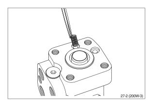
(41) Screw in the two setting screws using a 6mm hexagon socket spanner. Make the pressure setting on a panel or the machine.
