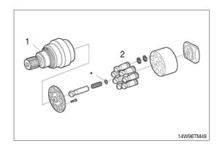
(1) Remove fixing screw (cylinder). Remove cylinder.
