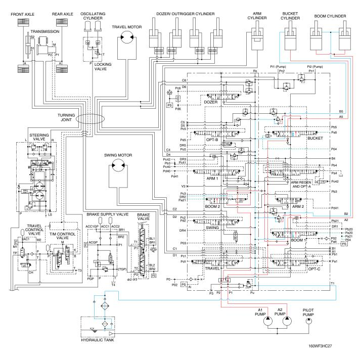
When the boom up and bucket in function are operated simultaneously, each spool in the main control valve is moved to the functional position by the pilot oil pressure from the remote control valve.
