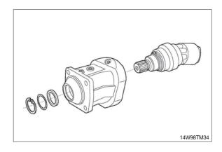
(1) Screw in threaded pin into center pin. Fix the cylinder with disc and locknut. M8 $\times$ 105 l
