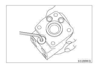
② Unscrew the setting screw using an 8mm hexagon socket spanner.
