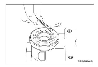
(18) Screw the threaded bush lightly into the check valve bore. The top of the bushing must lie just below the surface of the housing.
