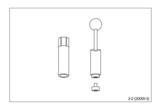
(3) Assembly tool for cardan shaft (11).
