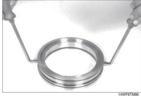
23) Remove seal and O-rings (see arrows) from pressure ring and ring.
