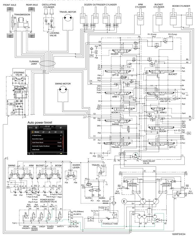
When the power boost switch on the left remote control lever is pushed ON, the power boost solenoid valve is actuated, the discharged oil from the pilot pump flows into **Pu** port of the main relief valve in main control valve; then the setting pressure of the main relief valve is raises from 350 kgf/cm² to 380 kgf/cm² for increasing the digging power. And even when press continuously, it is canceled after 8 seconds.
