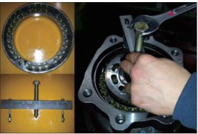
⑤ Disassemble respectively cylinder block sub (8), friction plate (13), separate plate (14) from casing (1).
