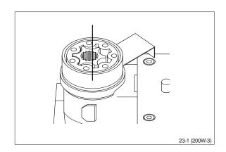
(27) Fit the gearwheel (rotor) and cardan shaft so that a tooth base in the rotor is positioned in relation to the shaft slot as shown. Turn the gear rim so that the seven through holes match the holes in the housing.
