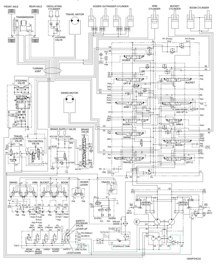
When the lever of the safety solenoid valve is moved upward, oil flows into the remote control valves through solenoid valve and line filter.
