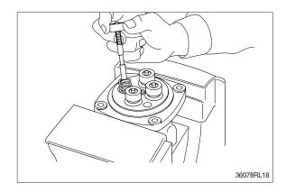
(3) Assemble O-ring (10) onto plug (8).
