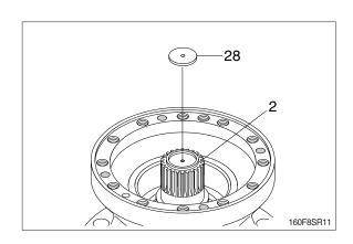
(11) Remove drive shaft (2) with roller bearing(3) and oil seal (4) assembled.Remove knock pin (29) from the casing (1).
