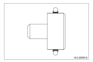
(12) Hole the outer part of the assembly tool in the bottom of the steering unit housing and guide the inner part of the tool right to the bottom.
