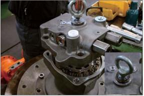
Assemble level gauge (42) into body (1).
