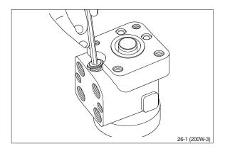
(38) Screw plug with dust seal into the housing using an 8mm hexagon socket spanner.
