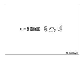
⑤ The steering valve is now completely disassembled.
