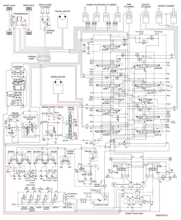
When the brake pedal (valve) is pushed, the discharged oil from the power train pump (P2) flows into the front and rear axle brake piston through the solenoid valve of brake supply valve. This pressure is applied to axle brake disc, thus the service brake is applied.
