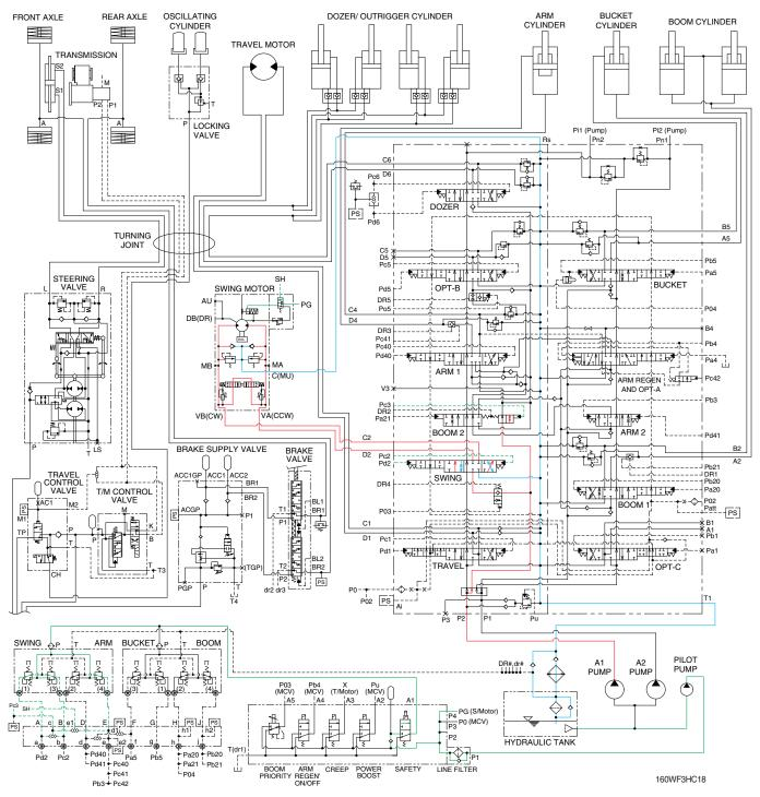
When the left control lever is pushed left or right, the swing spool in the main control valve is moved to the left or right swing position by the pilot oil pressure from the remote control valve.
