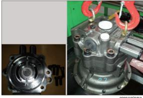
① Disassemble spring (16) and using a jig, disassemble parking piston (15) from casing (1).
