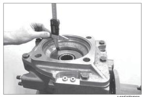
38) Determine Dim. C (Measuring hole II) from mounting face/housing to front face/piston (brake).
