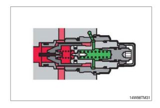
(3) Remove counter-balance valve. Inspect O-ring
