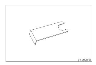
(4) Assembly tool for dust seal (1).
