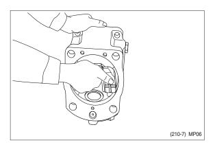
(12) Tapping lightly shaft ends of drive shafts (111, 113) with plastic hammer, take out drive shafts from swash plate supports.
