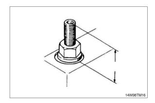
(2) When tightening, counterhold setting screw, then check setting height.
