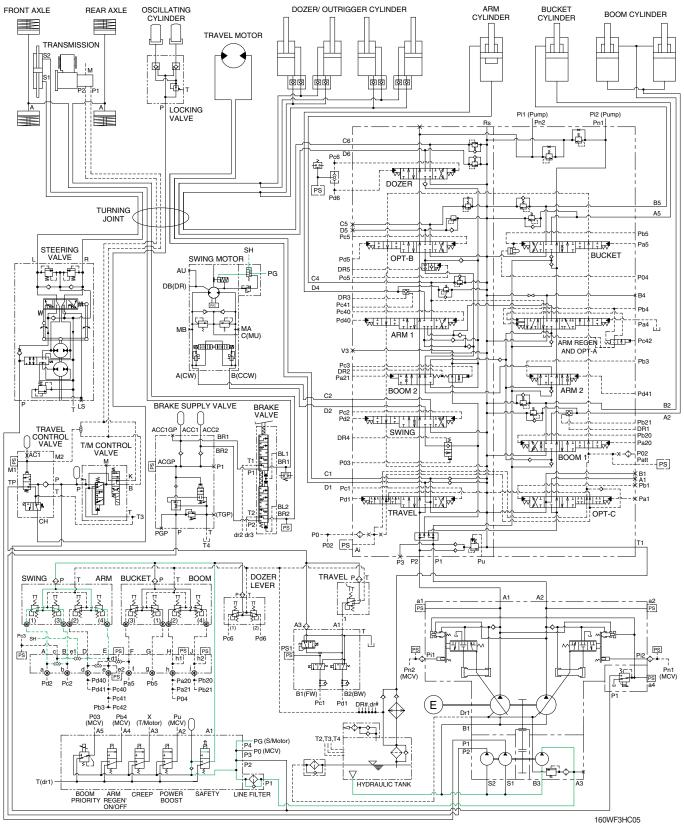
When the swing control lever or arm in control lever is tilted, the pilot oil flows into SH port through the terminal block. This pressure move spool so, discharged oil from pilot pump flows into swing motor PG port.
