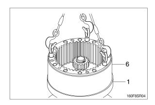
(12) Hammer 4 knock pins (29) around the ring gear (6).
