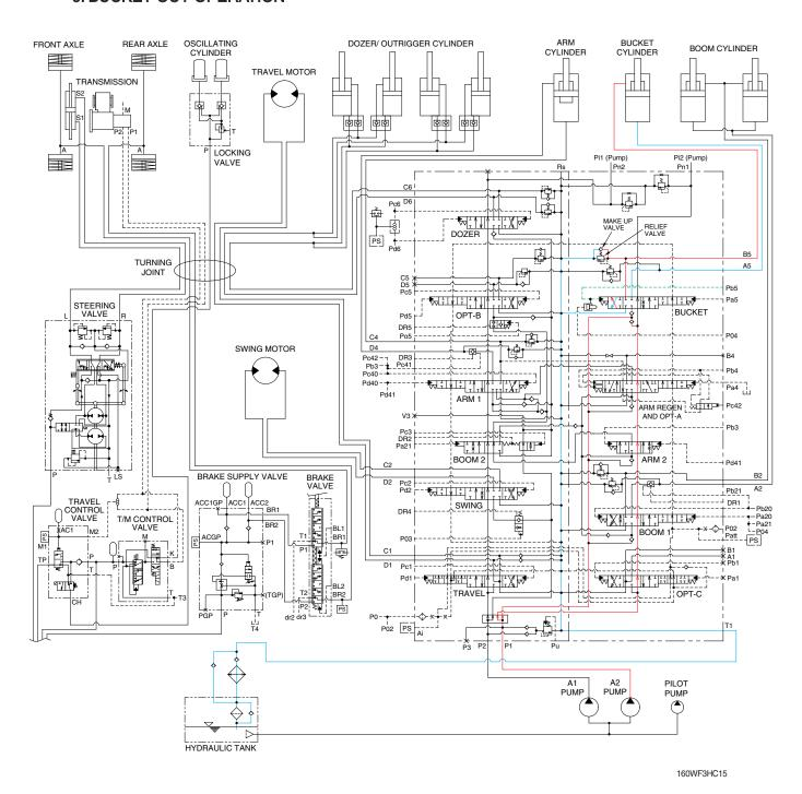
When the right control lever is pushed right, the bucket spool in the main control valve is moved to the bucket out position by the pilot oil pressure from the remote control valve.
