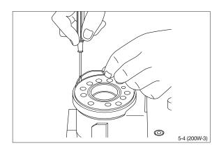
(8) Shake out the check valve ball and suction valve pins and balls.
