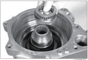
20) Remove pressure piece and compression spring.
