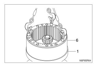
(4) Remove sun gear1 (22) from side plate 3 (19).
