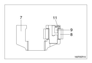
(5) Assemble carrier 2 (7) assembly correctly to the drive shaft (2).
